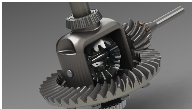
Figure 2-5: Open differential with pinion and ring gears. Reproduced as is from [19].
