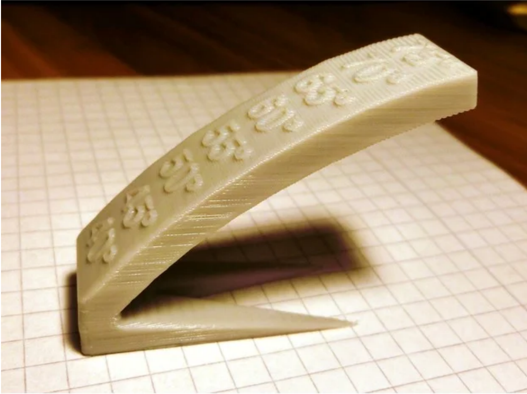
Figure B-11: 3D Printing Overhangs. (Reproduced as is from [83]).
