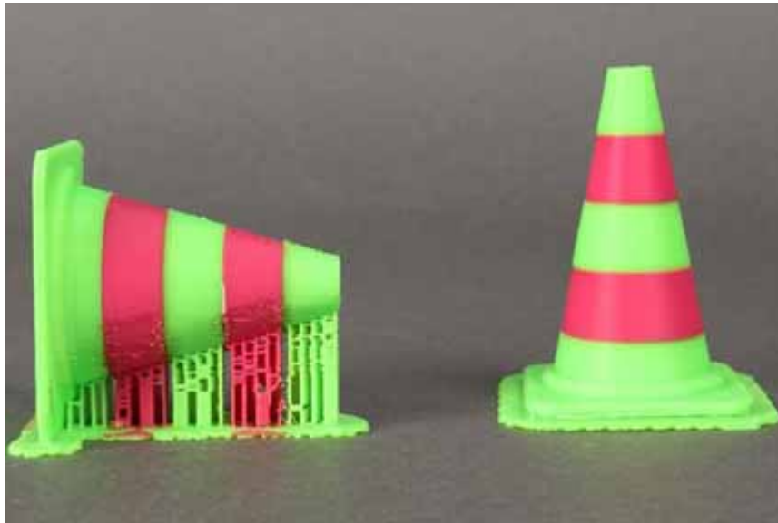
Figure B-10: 3D Printing Orientation. (Reproduced as is from [83]).
