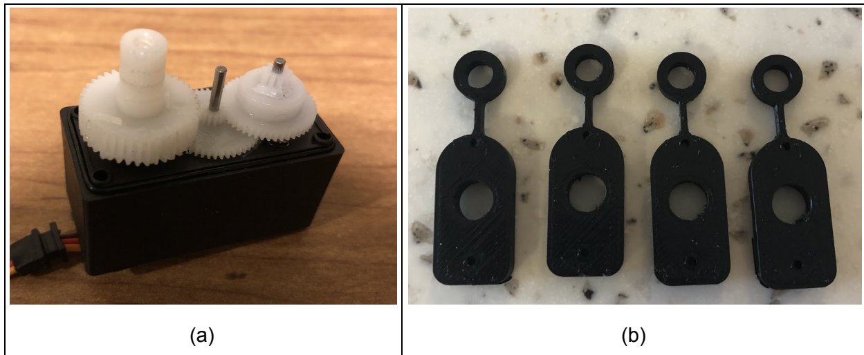
Figure 4-17: Steering assembly failures of test car, servo with stripped gears (a) and replacement steering link (b).
