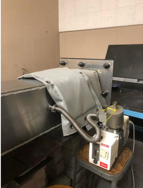
Figure C3: Collimator covered in Pb blankets to shield from unwanted radiation
