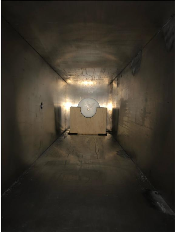
Figure C2: PE moderator with wooden stands placed inside of vacuum chamber
