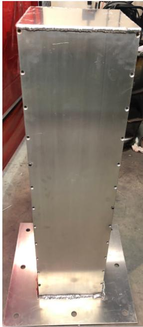
Figure 13: TIG welds on vacuum chamber
