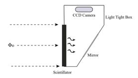
Figure 5: Neutron imaging camera setup [12]
