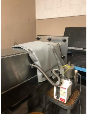
Figure C3: Collimator covered in Pb blankets to shield from unwanted radiation
