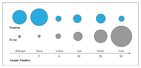
Figure 2: Relative probability of attenuation for X-rays and neutrons [2]
