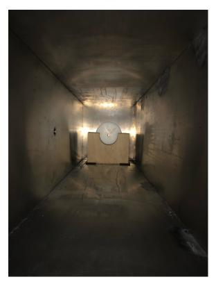
Figure C2: PE moderator with wooden stands placed inside of vacuum chamber
