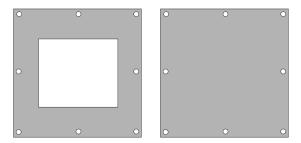
Figure 8: Vacuum chamber end plates
