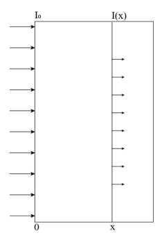
Figure 1: Beam intensity throughout a material [5]
