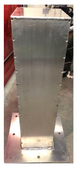
Figure 13: TIG welds on vacuum chamber
