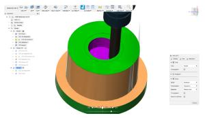
Figure 6: CAM simulation for convergent moderator
