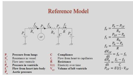
Figure 74. Reference model with all variables for the heart simulation
