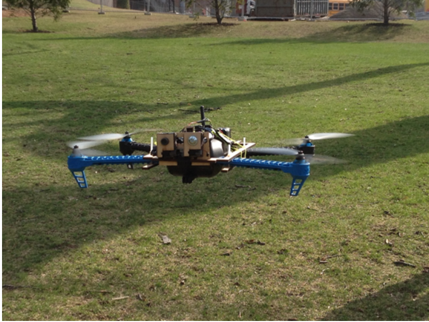
Figure 1: Our fully-assembled depth-mapping system in flight.
