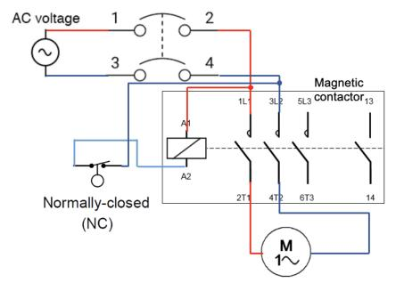
Electrical diagram for auto-emptying and auto-filling a tank
