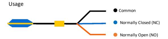
Depending on the mode selected, a float switch can either turn the circuit on or off at its up position. This is called normally open and normally closed, respectively.
