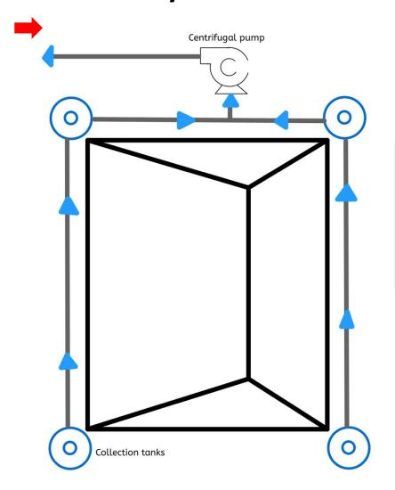
The connecting pipes in each tank should be placed at the bottom of the tanks with return valves to avoid the water from flowing back.
