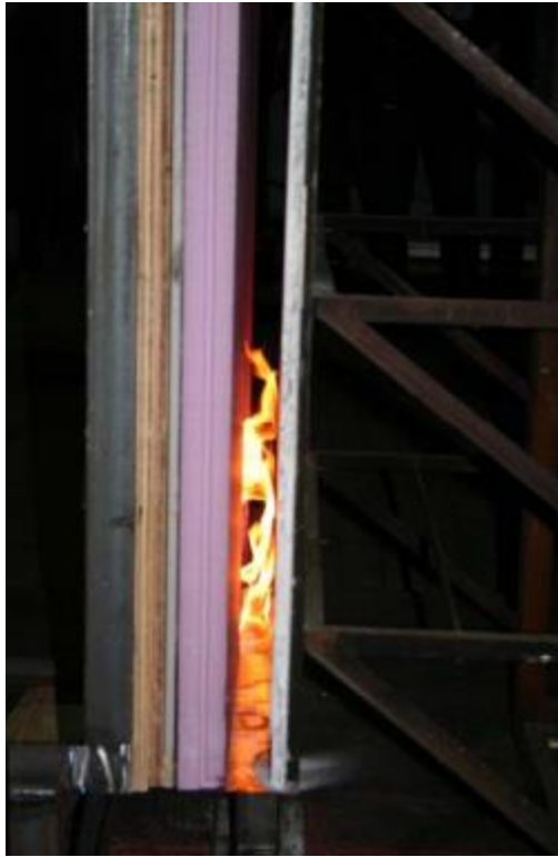
Figure 17: An image of test FM 4411 being conducted (32)
