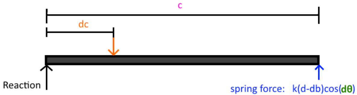
Figure 17: FBD of ramp treated a cantilever beam
