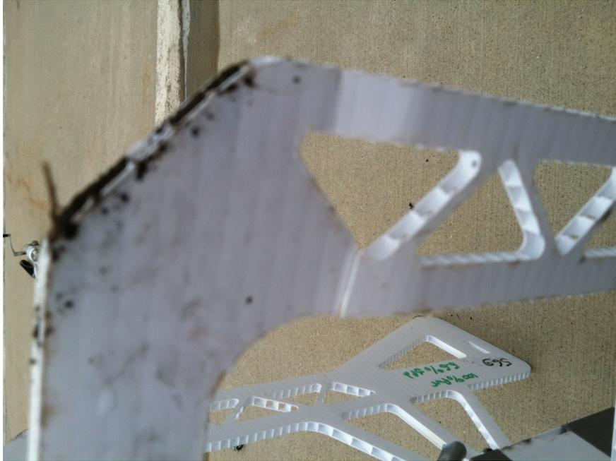
**Figure 105:** Damage sustained from the drop test
