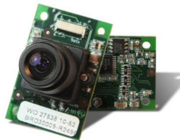
**Figure 58:** The Caspa camera module [22]
