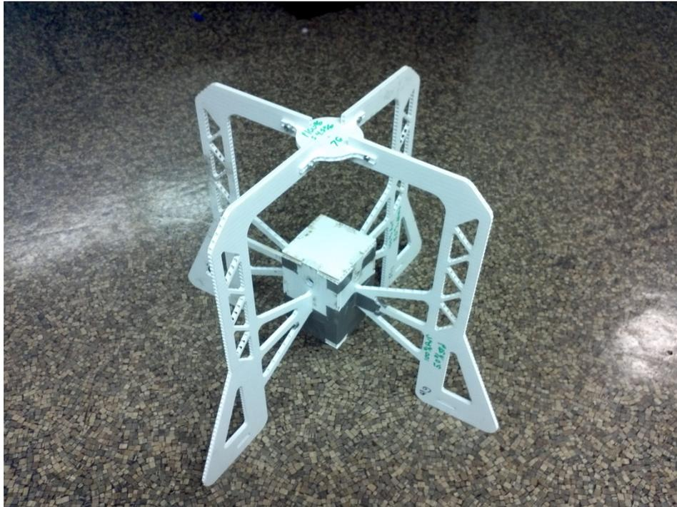
**Figure 103:** Chassis used in the drop test
