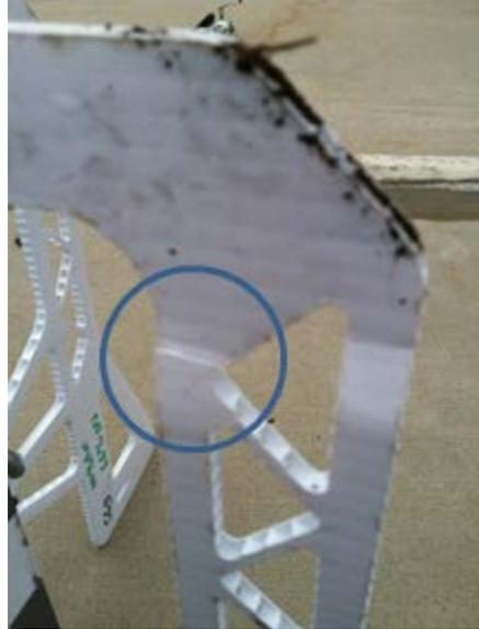
**Figure 28:** Close up of damage after impact, notice the cracked plastic in the circle
