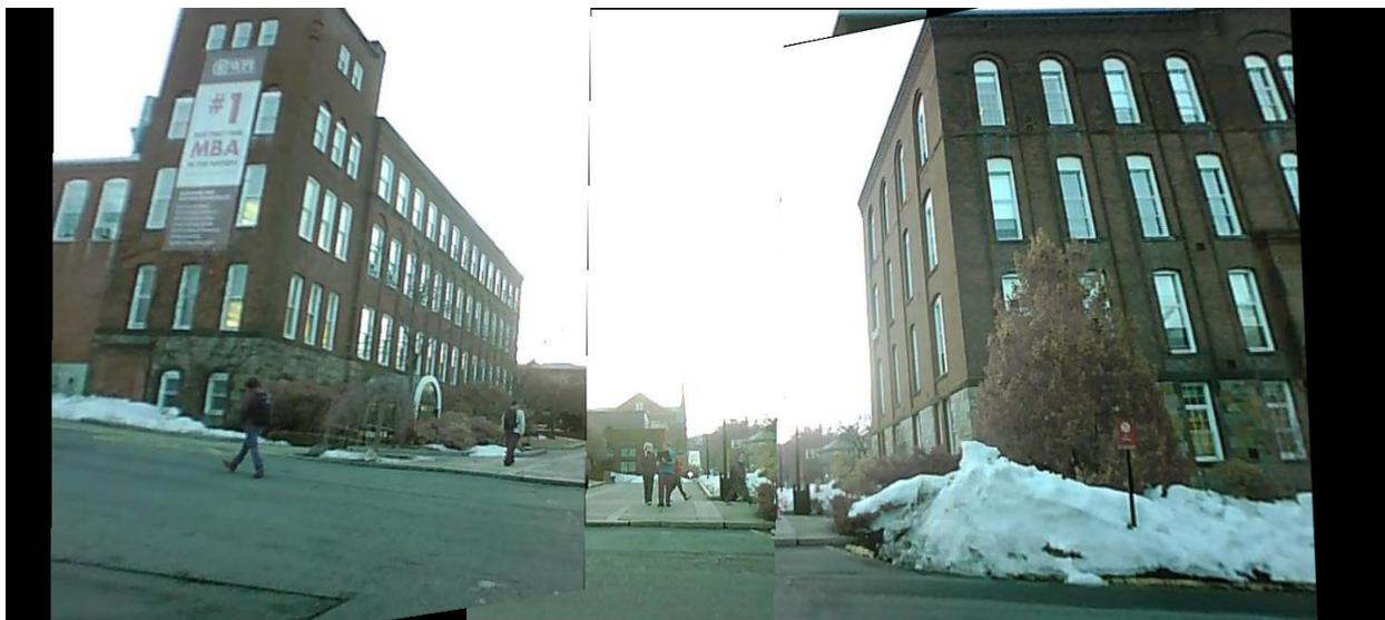
**Figure 96:** Stitching offset caused by camera lens movement.
