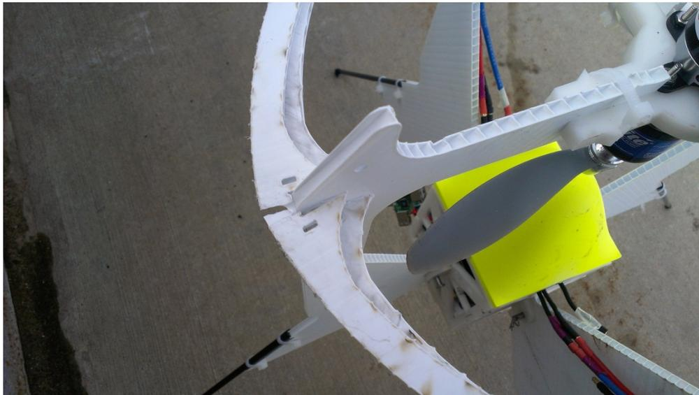
**Figure 133:** Damage to the propeller protection ring
