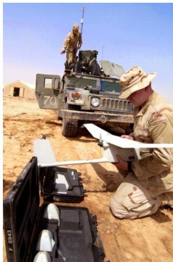
**Figure 5:** The RQ-11 Raven being assembled before flight.
