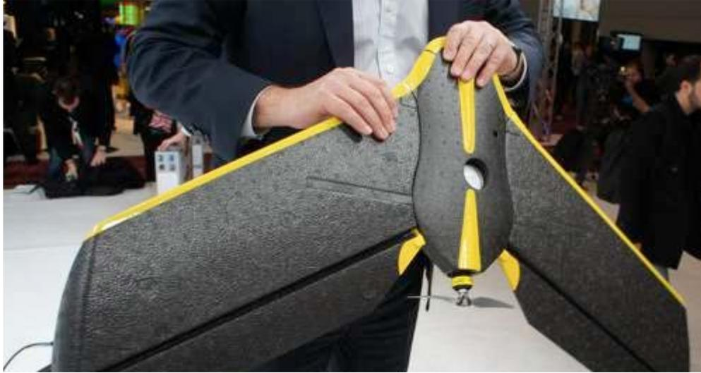
**Figure 7:** The eBee 3D mapping UAV [30]
