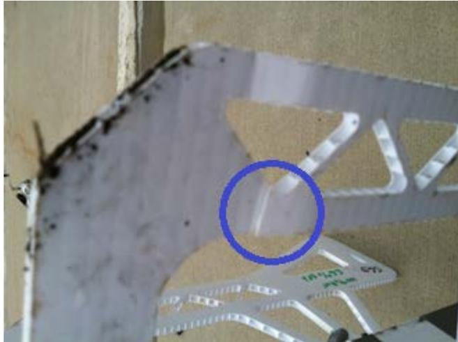
**Figure 23:** Details of chassis damage after drop test
