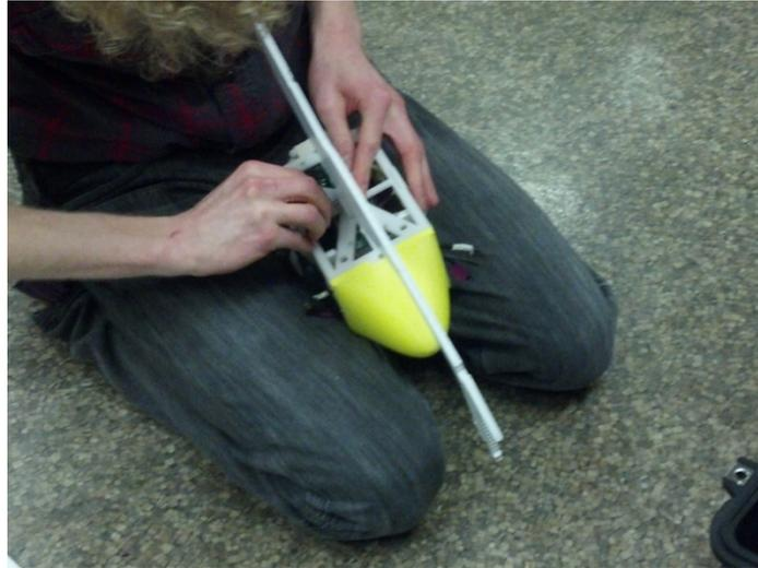
**Figure 144:** Affixing the panels to the electronic box with clevis pins
