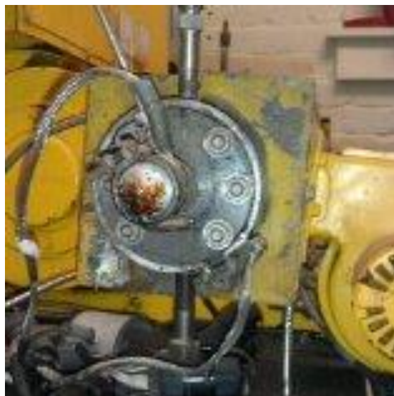
Figure 35 Die Bolted on
