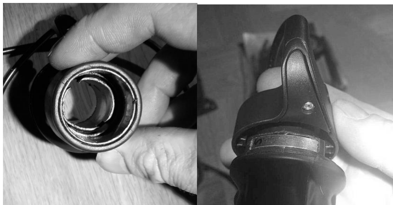
Figure 5. Half-twist grip hall sensor (Endless Sphere, 2016)
