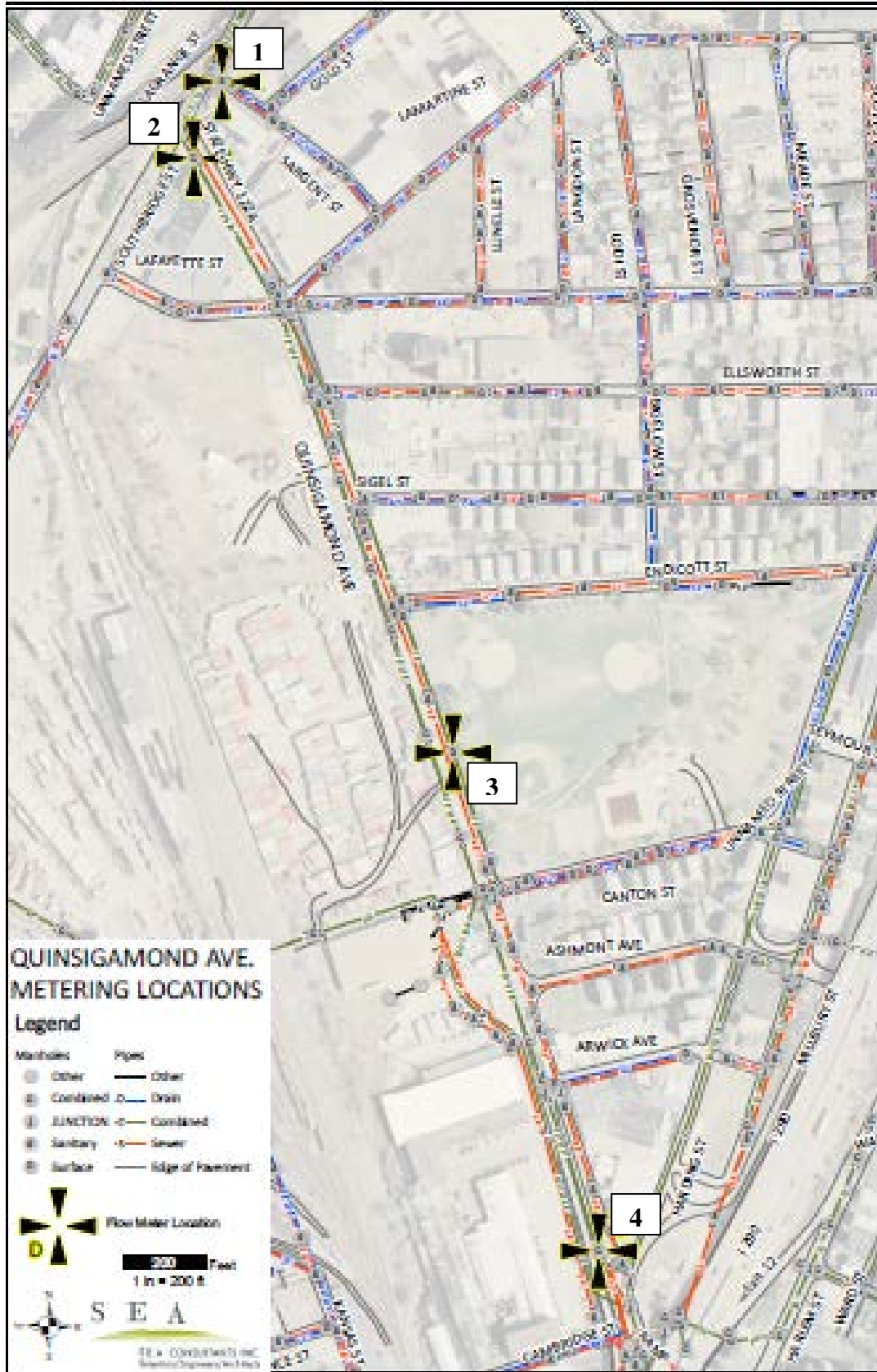
Figure 8: Flow Metering Locations (Kleinfelder/SEA, 2010)
