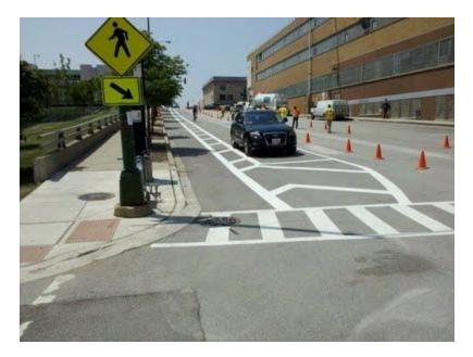
Figure 72 – Cycle Track (Burton) typical cycle track implementations consist of painted lines, designated areas for pedestrians, cyclists and parked motorists.
