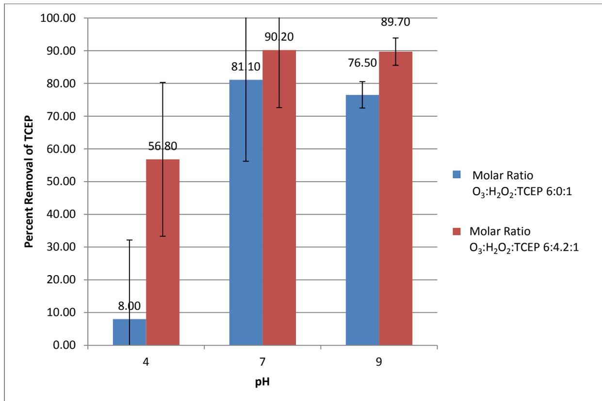
Figure 8: Percent Removal of TCEP for O<sub>3</sub> and H<sub>2</sub>O<sub>2</sub>/O<sub>3</sub> Treatments at Varied pH (Ozone Dose of 2 mg/L).
