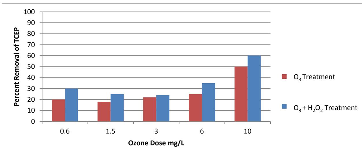
Figure 7: Percent Removal of 5000 ng/L TCEP by  $\text{O}_3$  and  $\text{H}_2\text{O}_2:\text{O}_3$  (0.7:1 molar ratio) Oxidation at pH 8.1 (Data from Pisarenko et al. 2011 [41]).
