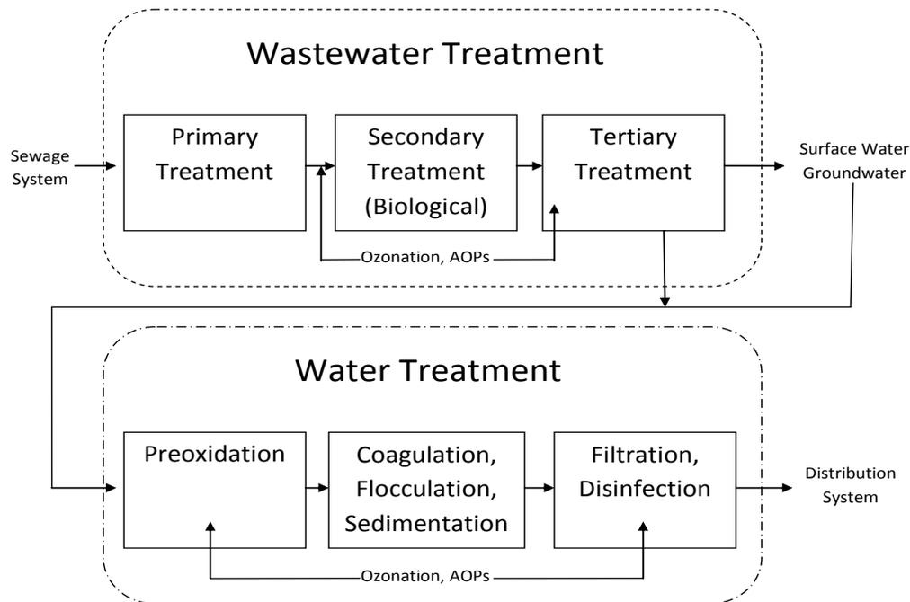
Figure 2: Potential Points to Apply Ozonation to Existing Water or Wastewater Treatment Plants
