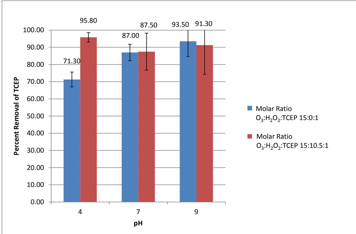
Figure 9: Percent Removal of TCEP for O<sub>3</sub> and H<sub>2</sub>O<sub>2</sub>/O<sub>3</sub> Treatments at Varied pH (Ozone Dose of 5 mg/L)
