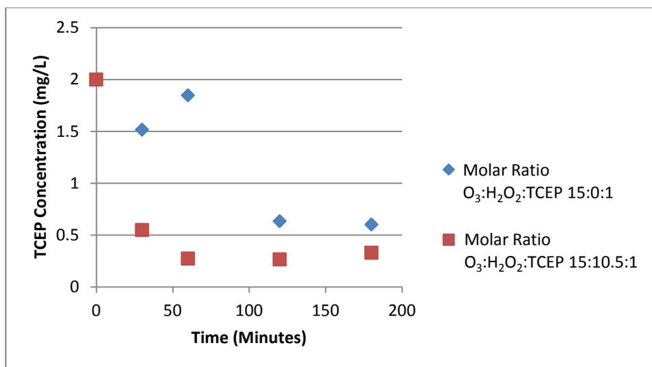
Figure 12: Kinetics Experimental Data for O<sub>3</sub> and O<sub>3</sub>/H<sub>2</sub>O<sub>2</sub> Oxidation of TCEP (pH = 7, Initial TCEP = 2 mg/L, Ozone Dose = 5 mg/L, and Hydrogen Peroxide Dose = 2.5)
