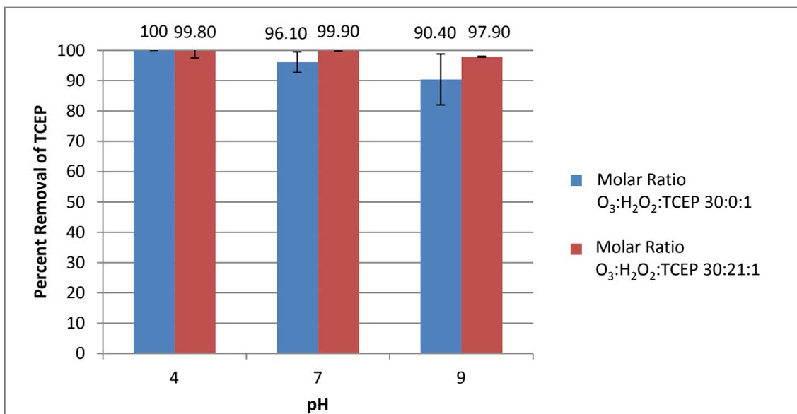
Figure 10: Percent Removal of TCEP for O<sub>3</sub> and H<sub>2</sub>O<sub>2</sub>/O<sub>3</sub> Treatments at Varied pH (Ozone Dose of 10 mg/L).
