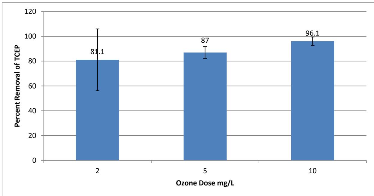
Figure 5: Effect of Ozone Dose on Ozone Oxidation of TCEP at pH 7.
