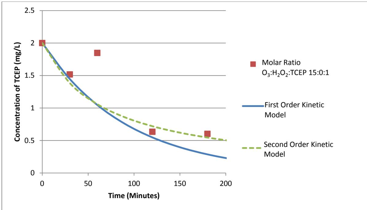
Figure 13: Measured and Kinetic Model Values of TCEP Concentration with Ozone Treatment. (Initial Conditions: TCEP = 2 mg/L, Ozone = 5 mg/L, Hydrogen Peroxide = 0 mg/L, pH = 7  $O_3:H_2O_2:TCEP$  Molar Ratio of 15:0:1).
