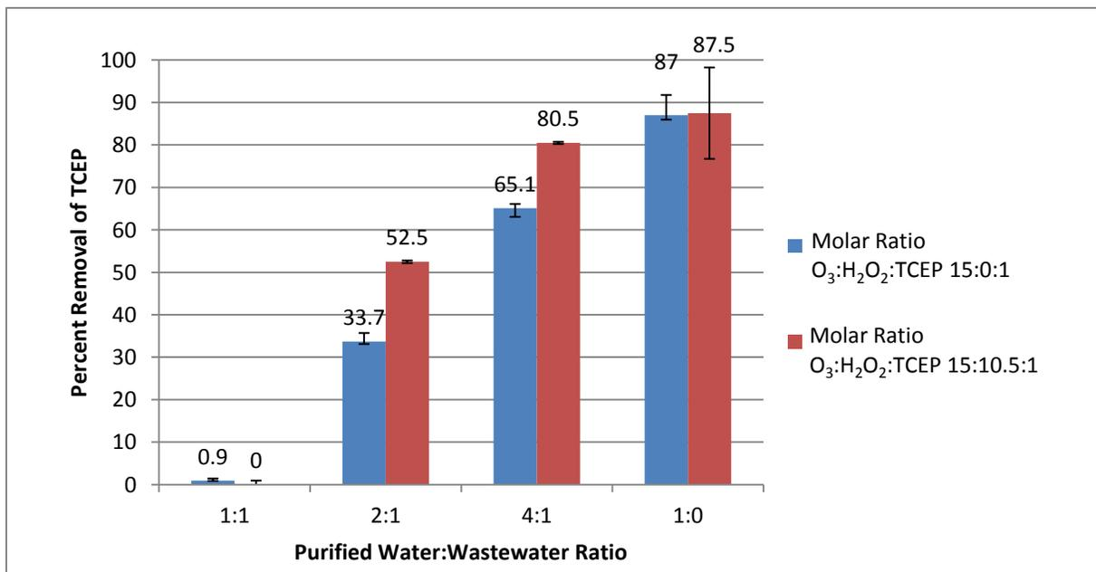
Figure 11: Percent Removal of TCEP for O<sub>3</sub> and H<sub>2</sub>O<sub>2</sub>/O<sub>3</sub> Treatments in Diluted Wastewater at pH 7 (Ozone Dose of 5 mg/L). Initial TCEP Concentration = 2 mg/L.
