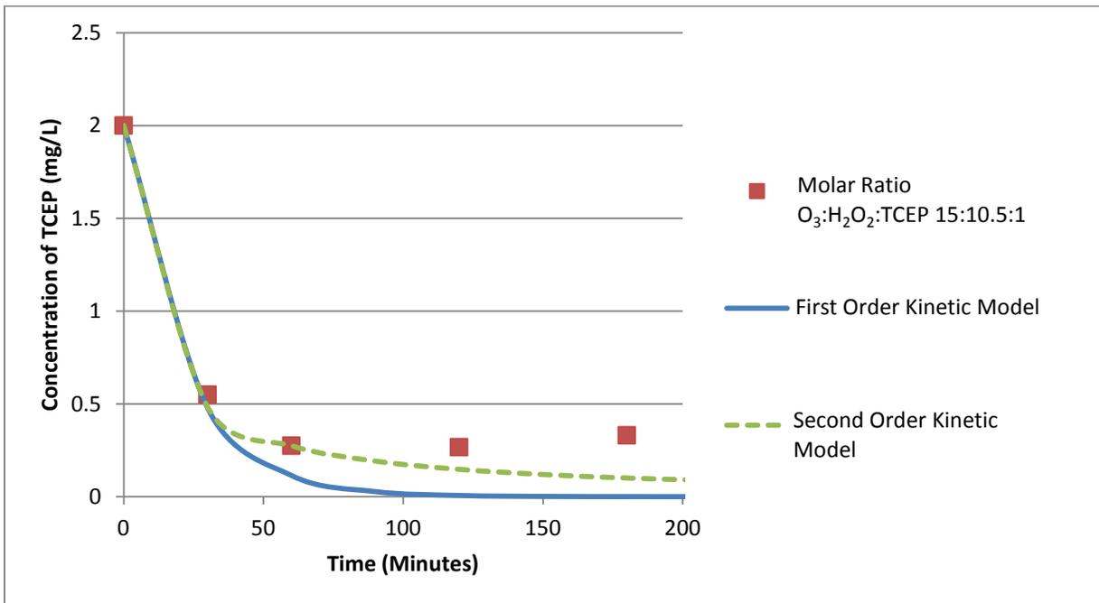
Figure 14: Measured and Kinetic Model Values of TCEP Concentration with Ozone/Hydrogen Peroxide Treatment.
