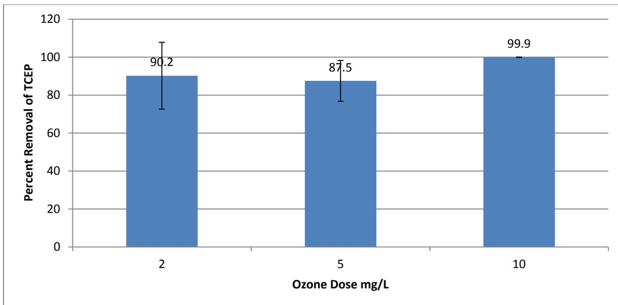
Figure 6: Effect of Ozone Dose on Ozone/Hydrogen Peroxide Oxidation of TCEP at pH 7 (Ratio of  $\text{H}_2\text{O}_2:\text{O}_3$  of 0.5:1 by mass). Initial TCEP Concentration = 2 mg/L.
