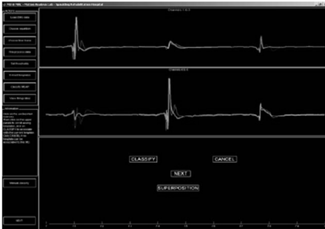
Figure B.11: A motor unit that has been classified manually (colored). The template which matches the motor unit shown in white. This template is composed of six waveforms from across all channels.
