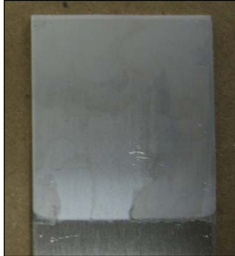
Figure 25: Residue that Remained on Specimen
