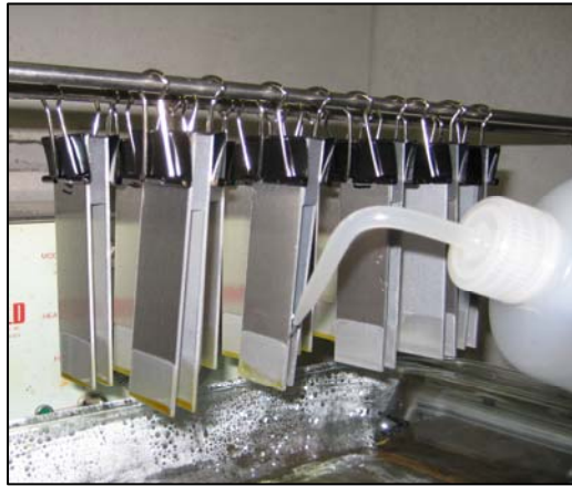
Figure 18: Spraying of De-Ionized Water on Treated Specimens
