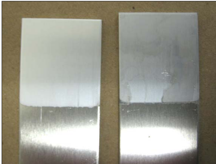
Figure 27: "New" Cleaning Method (right) vs. "Old" Cleaning Method (right)
