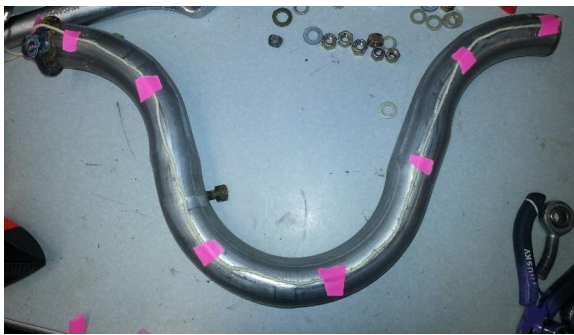
Figure 155: Exhaust Header Pipe
