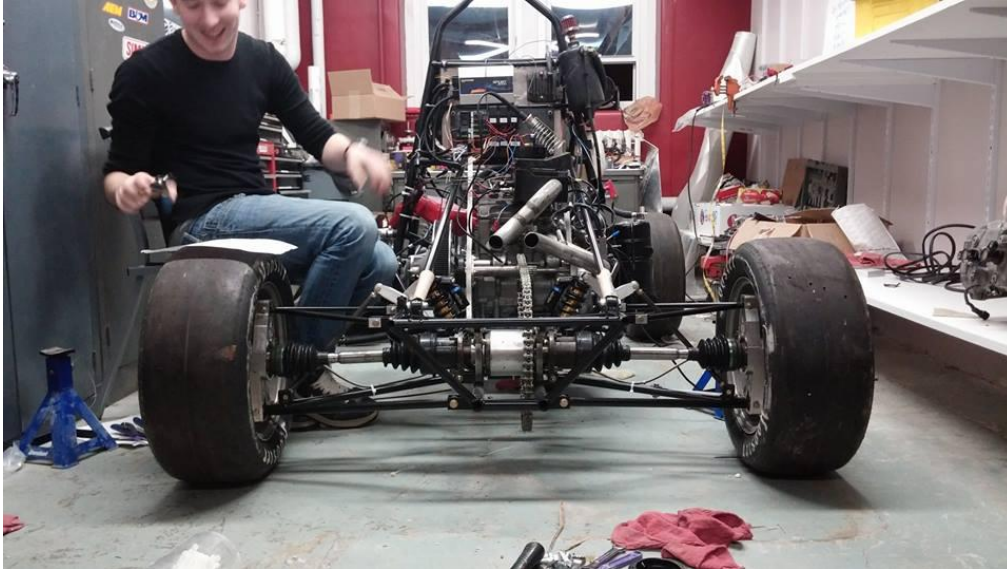
Figure 61: Suspension at Ride Height
