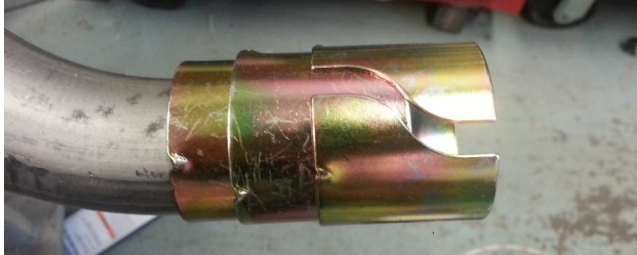
Figure 158: Reducer on the Header Pipe
