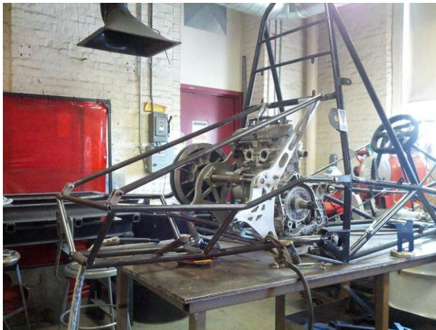
Figure 36: Welding of Subframe
