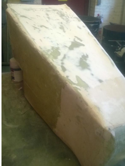
Figure 152: Filled Surface Defects
