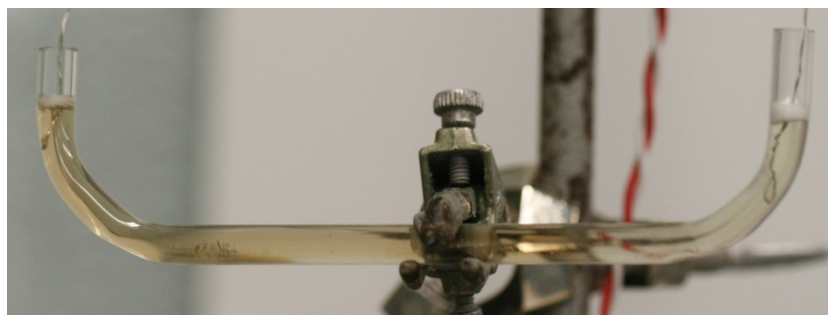
Figure 77: Observation 2 Full Tube: Color gradient darkening from cathode to anode, protein accumulation near the bend towards the anode electrode
