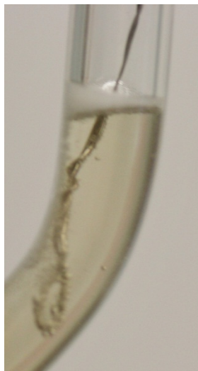
Figure 74 - Observation 1 Cathode: Fizzing on electrode
