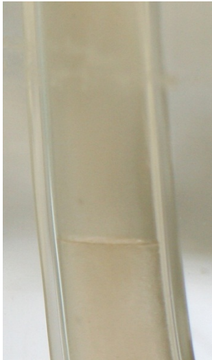
Figure 58 - Observation 3 Anode Interface: Clear band above interface continues to grow
