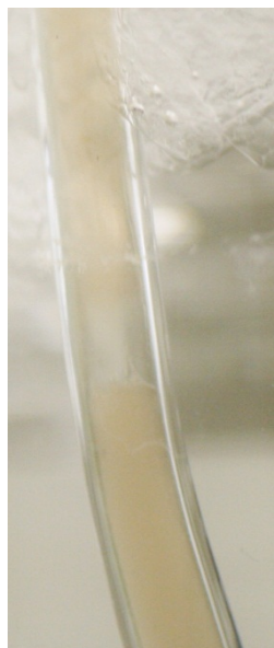
Figure 52 - Observation 1 Anode Interphase: Formation of clear band beneath the interface as protein migrates towards the cathode
