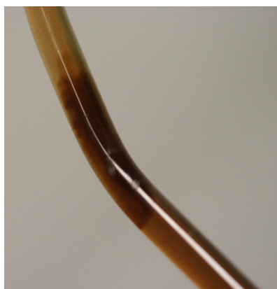
Figure 36 - Observation 2 Protein Accumulation: The protein accumulation continued to rapidly migrate further into the bottom phase towards the cathode
