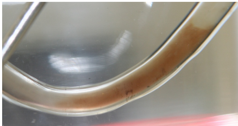
Figure 61 - Observation 5 Protein Accumulation: Continued, yet slowed migration of protein towards the cathode
