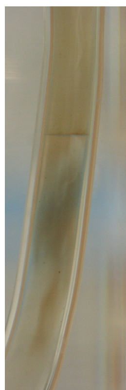
Figure 69 - Observation 2 Cathode Interphase: Protein continues to diffuse through interface boundary
