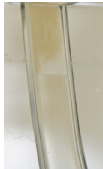
Figure 64 - Observation 1 Anode Interface: Protein migration away from interface towards electrode
