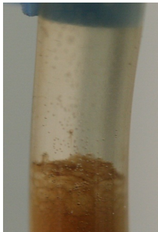
Figure 28 - Observation 3 Anode Interphase: Continued disruption of interface
