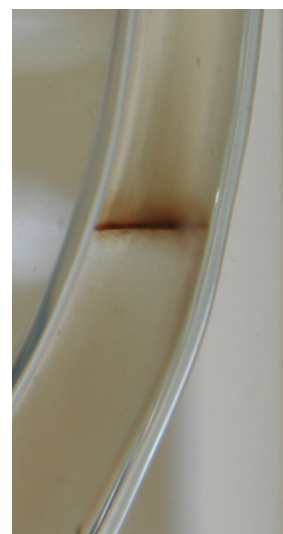
Figure 54 - Observation 2 Cathode Interface: Dark band at interface has grown more intense
