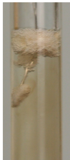
Figure 67 - Observation 2 Anode Electrode: Small white formation of protein precipitate on the electrode tip, larger formation of released protein at the surface of the top phase
