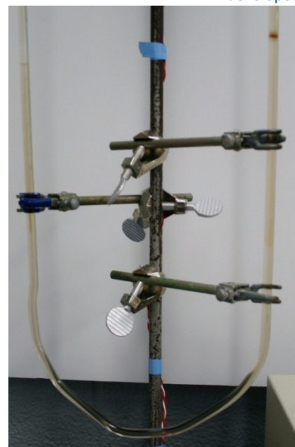
Figure 17 - Observation 6 Full U-Tube: Both interfaces can be seen near the top of the frame, the anode (left) appears clear above and dark below, while the cathode exhibits a dark band
