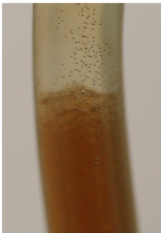
Figure 26 - Observation 1 Anode Interphase: Slight disruption of interface
