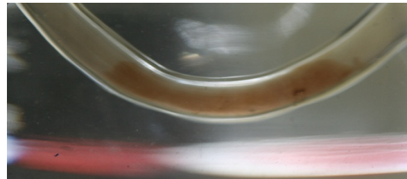
Figure 59 - Observation 4 Protein Accumulation: Cloud continues to migrate towards cathode
