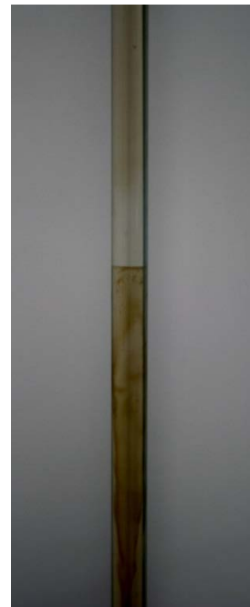
Figure 15 - Observation 5 Anode Interface: Diffusion of protein into bottom phase is much more prevalent and well developed
