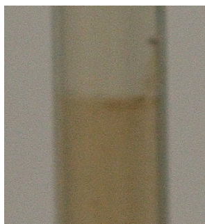
Figure 19 - Observation 1 Anode Interphase: Small concentration of protein beneath the interface
