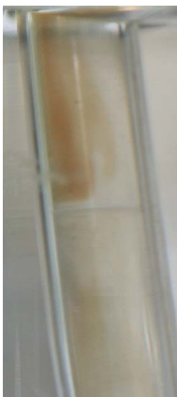
Figure 68 - Observation 2 Anode Interphase: Migration of protein through and away from interface towards anode electrode
