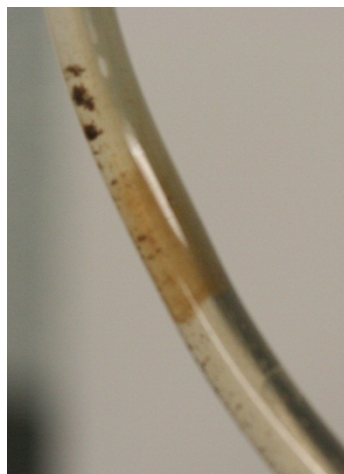
Figure 43 - Observation 1 Protein Cloud: Formation of a protein rich region in the anode side of the lower portion of the single phase
