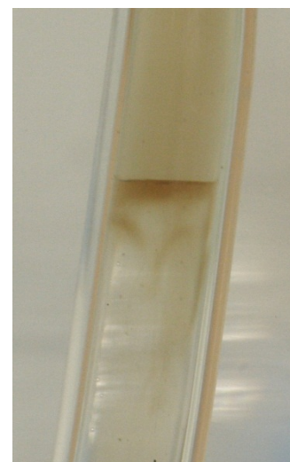
Figure 66 - Observation 1 Cathode Interface: Diffuse dark band below interface formed as protein migrates through interface
