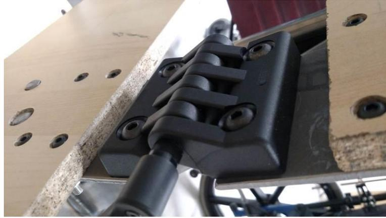
**Figure 43: Hinge Assembly connecting front board and thigh board.**
