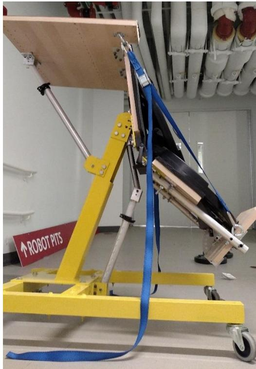
**Figure 48 Device showed no signs of risk or danger when loaded with weight plates adding up to 120 lbs. for an hour**
