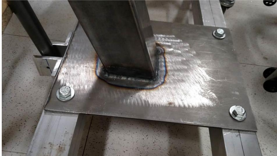
**Figure 40: Base Plate Assembly.**
