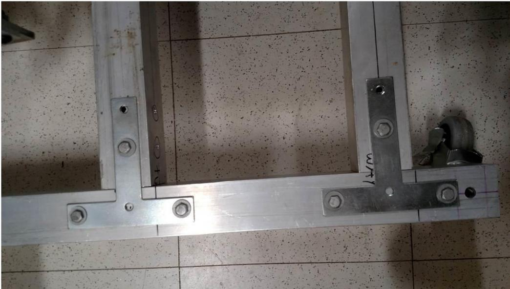
Figure 39: T-Bracket Assembly.
