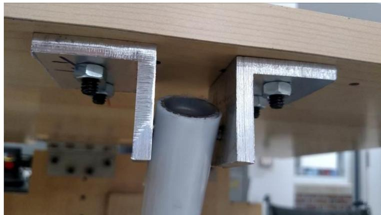
**Figure 47: L Brackets and Tray Connection.**
