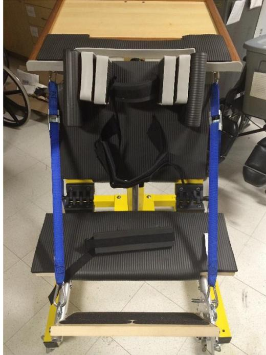
**Figure 46 Lateral Supports to Secure User**
