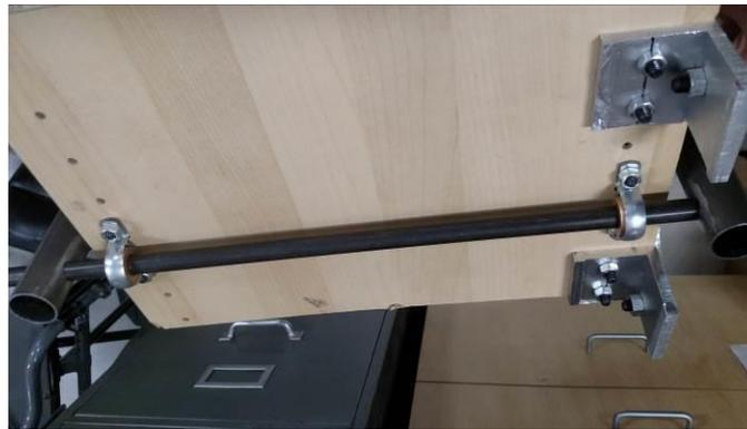
**Figure 44: Underside view of bearing assembly responsible for supporting footboard.**
