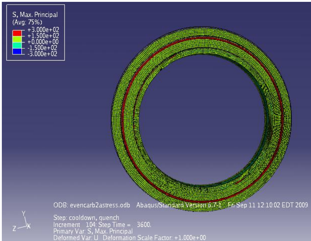
Figure 31: Maximum Principal Stresses for Evenly Quenched Simulation
