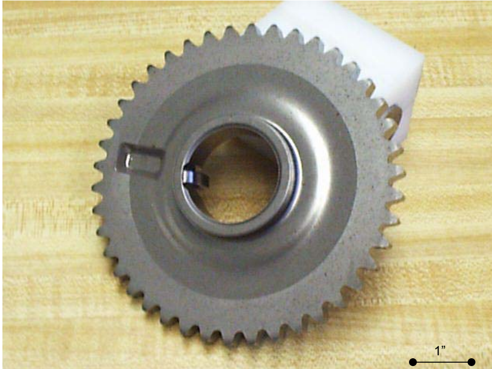
Figure 2.4: Complex, multi-level P/M part (courtesy of BorgWarner).
