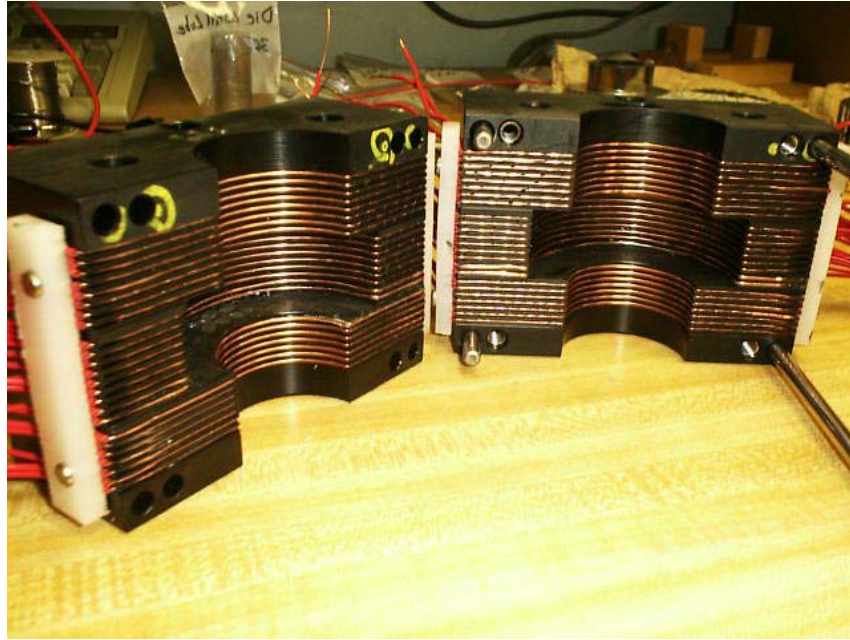
Figure 6.23: Sensor developed for measuring density in complex hub-shaped gear.
