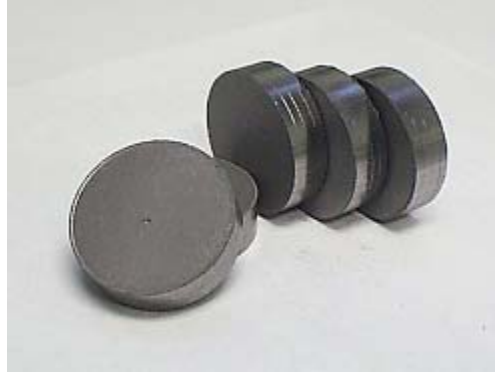
Figure 4.1: Controlled green-state P/M compacts used for the conductivity measurements.
