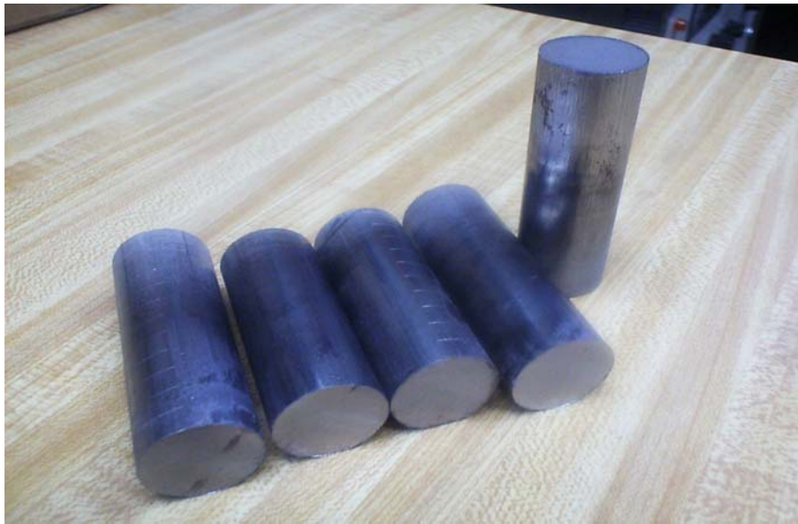
Figure 6.1: Green state P/M samples of length of 3" with length-to-width ratio of 4:1, used for measurement of density gradient.
