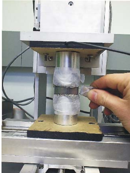
Figure 4.3: Semi-automated measurement setup for extended conductivity measurements.
