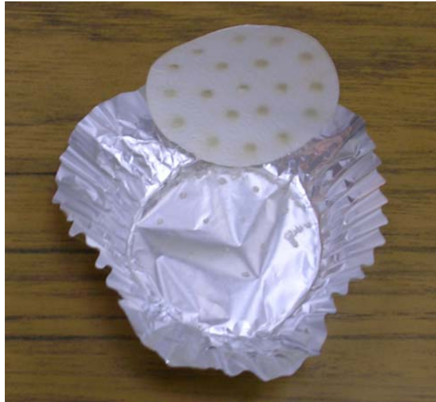
Photograph 12: Glass filter and aluminum dish after the reservoir total suspended solids test
