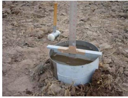
Photograph 11: Percolation test at Block3
