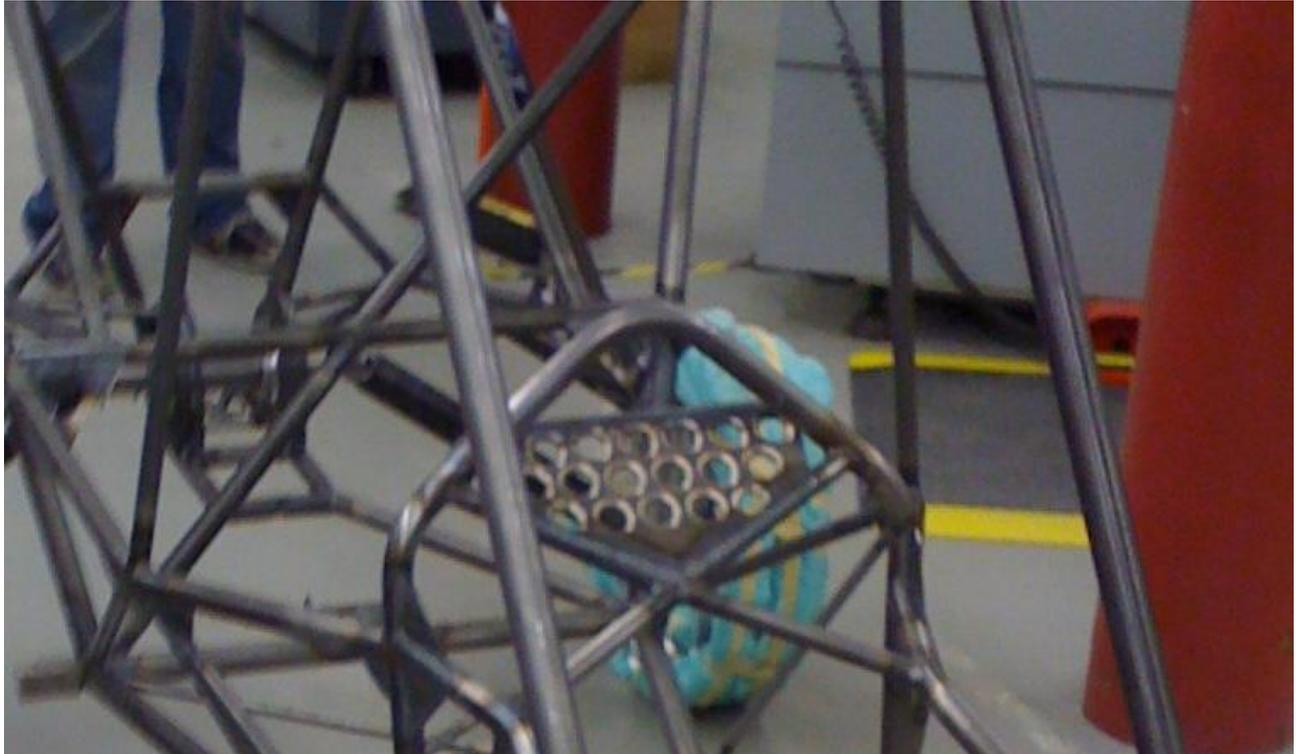
**Figure 8: Flared Hole Steering Column Mount**
