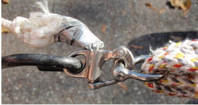
Figure 66: Release Mechanism
