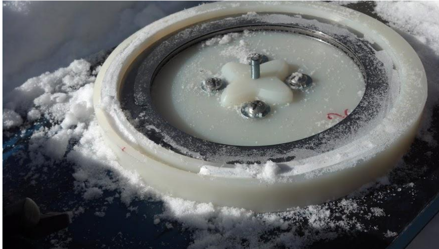
Figure 35: Snow Accumulation in Bearing Encasement
