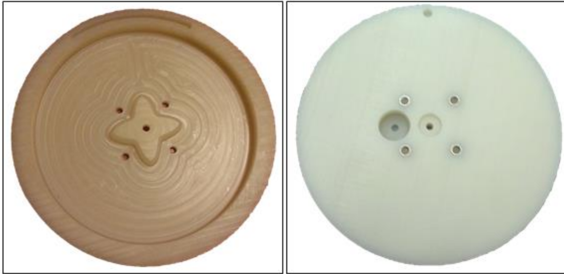
Figure 17: Machined Top (Right) and Bottom (Left) Plates
