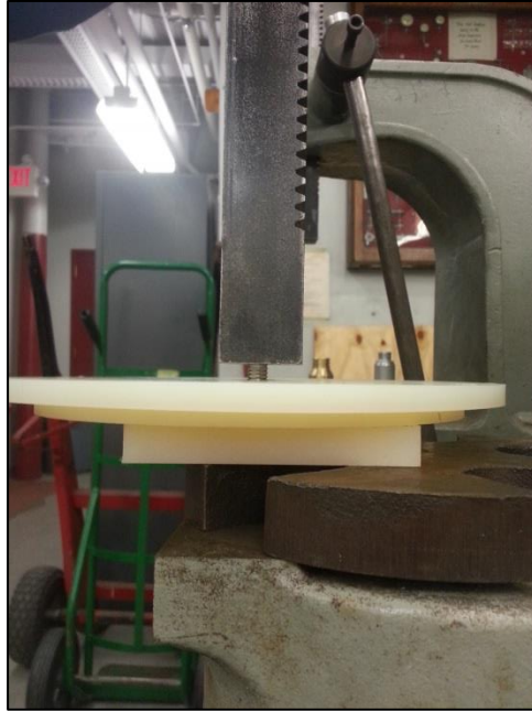
Figure 18: Press Fit of Threaded Inserts
