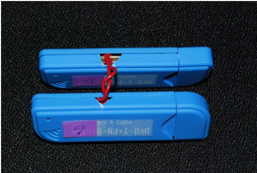
Figure 25 – Modified Two-Channel RTL-SDR with Casing
