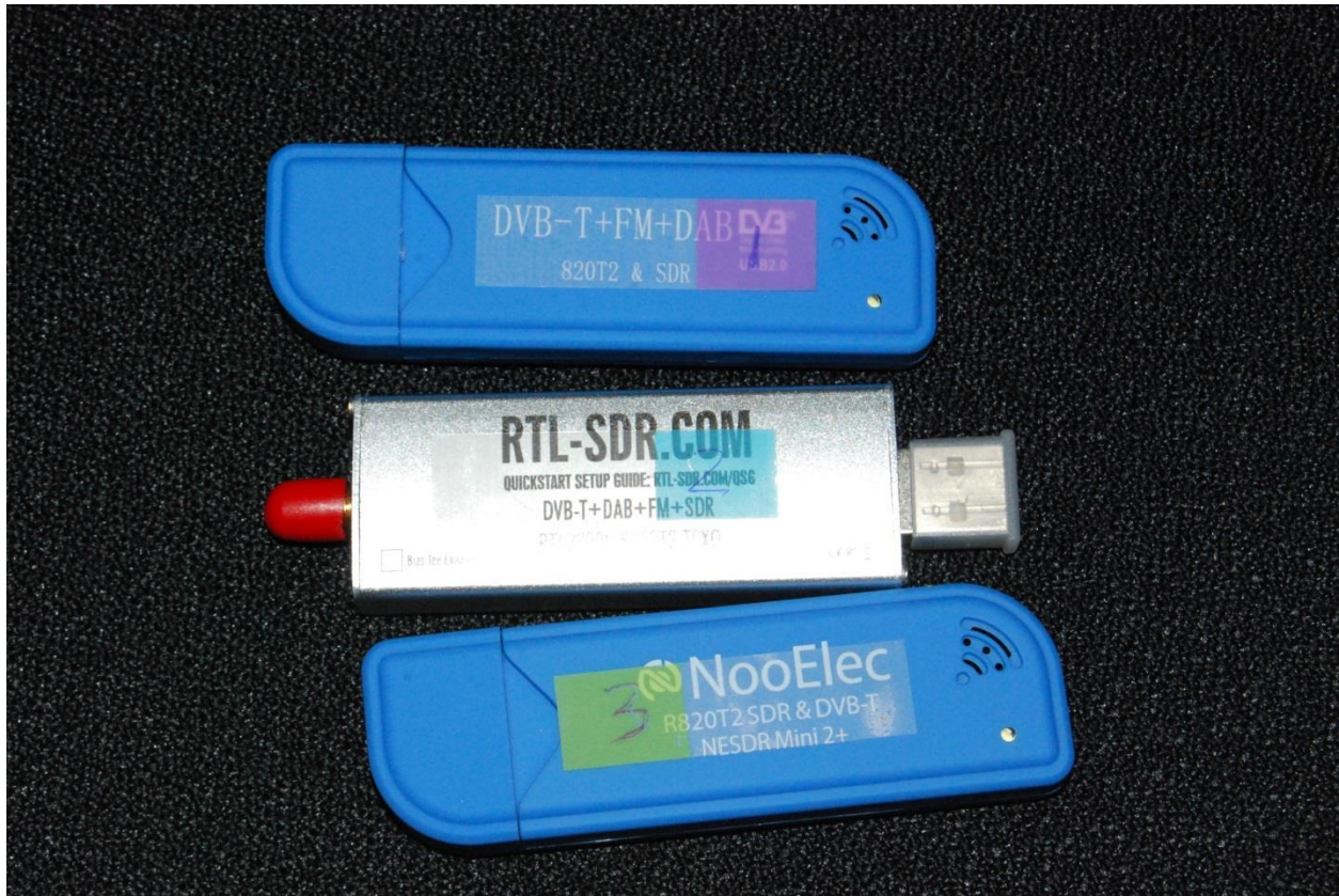
Figure 5 – Three RTL-SDR models. SQdeal RTL-SDR, RTL-SDR Blog RTL-SDR, and NooElec RTL-SDR, from Top to Bottom.
