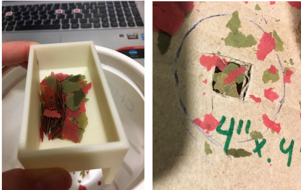
Figure 25: Flakes Clogging in 3D-Printed Reservoir (Left) and during Cardboard Test (Right)
