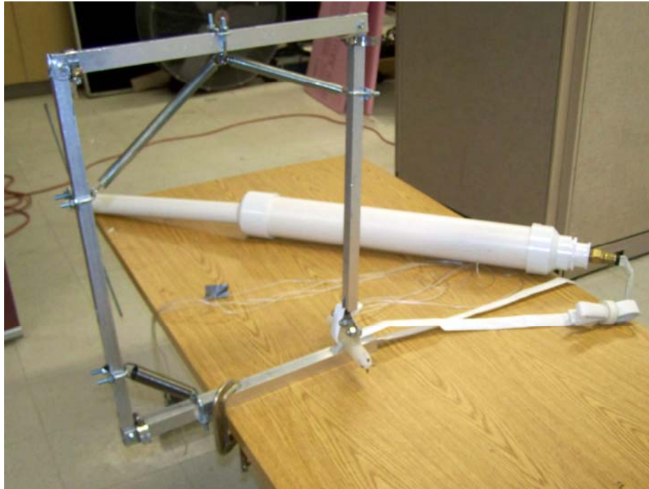
Figure 33 - Retracted assembly: With the plunger of the test pump in the depressurized position, the springs force the arm to fold and retract.
