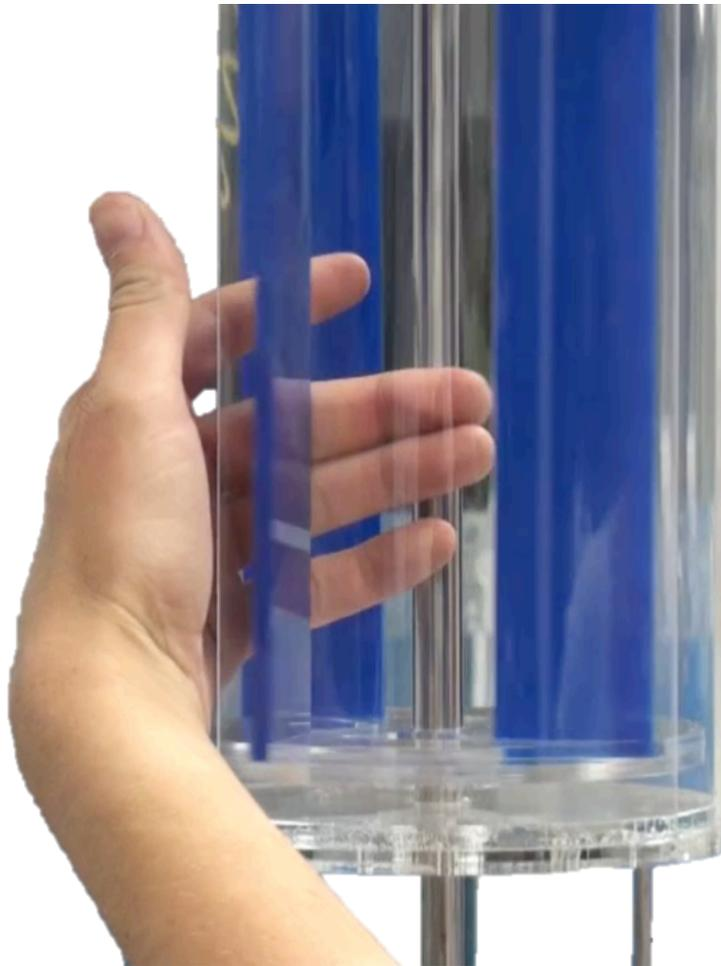
Figure 6. A detailed view of the four-bladed flat plate turbine with an angle of attack of 45° in enclosure E1. The inlet of the clear acrylic enclosure is demonstrated.
