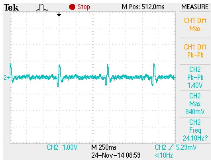
Figure 2.15: Three Electrodes Configuration Lead II
