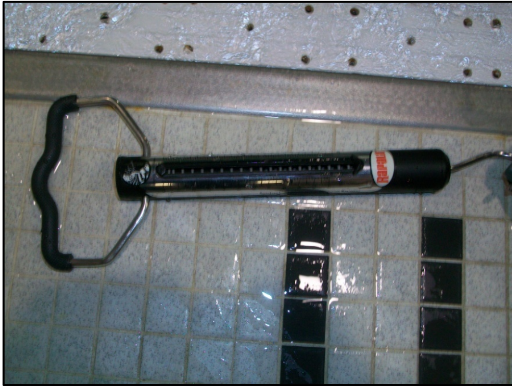
Figure 33: Rapala Spring Gage utilized during testing
