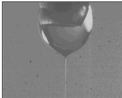
Figure 11: A stable Taylor cone; the top of the image is at the needle/droplet interface
