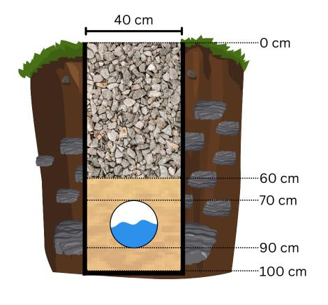
Using local costs in the village of Shtiqen, and the diagram as shown the following calculations were performed to achieve an estimate for the cost per linear meter.
