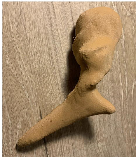
Figure 47: Malleus 3D printed from Polywood PLA
