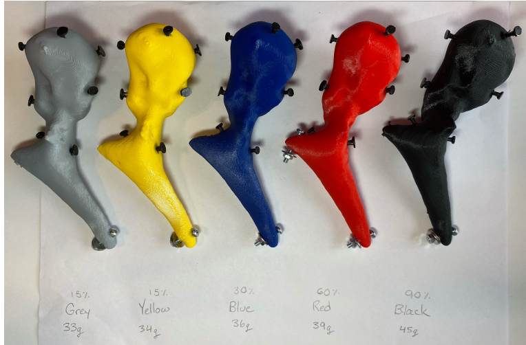
Figure 46: Malleus bones printed at various infills
