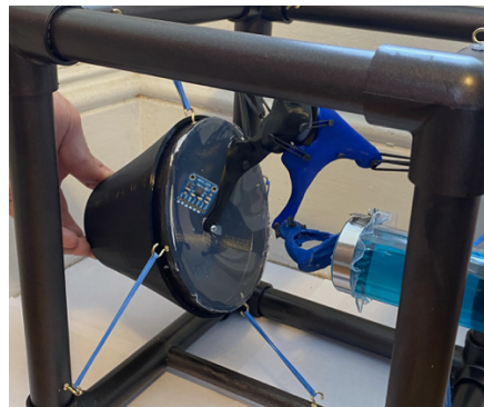
Figure 40: Accelerometer attachment to the tympanic membrane
