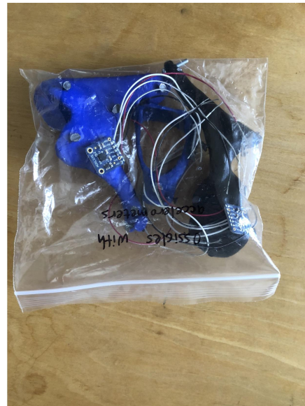
A set of ossicles with accelerometers attached:
