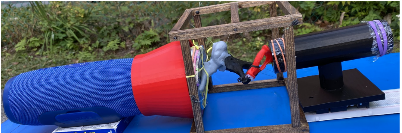
Figure 20: Initial cochlea print aligned with the first iteration prototype. The speaker, which is the blue, left most structure, was set up for acoustic stimulation.
