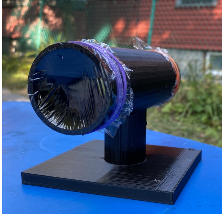
Figure 19: First 3D printed cochlea with transparent cling wrap ends
