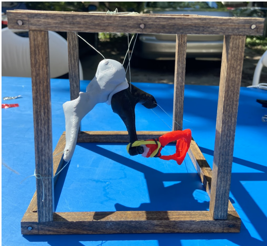
Figure 17: First rapid prototype involving 3D printed ossicles, moldable silicone joints, and rubber bands. The ossicles are as follows: grey = malleus; black = incus; red = stapes
