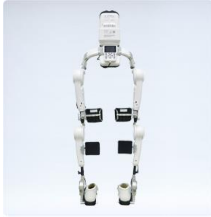
Figure 11: Cyberdyne's Hybrid Assistive Limb [29]
