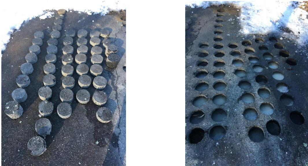
**Figure 4-5: Asphalt Cores from 2/26/ 2019 (Left) and Respective Asphalt Core Holes (Right)**
