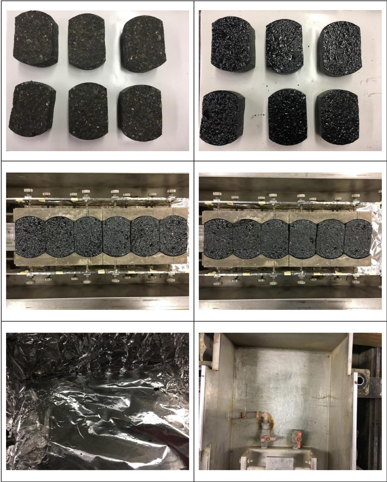
Figure C-3: Coal-Tar-Based, 48 Hours Cure Time, Test #1
