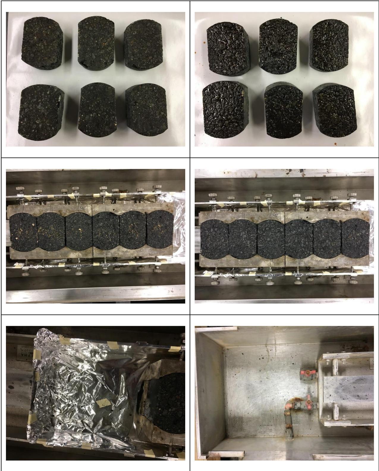
Figure C-15: Bio-Based, 48 Hour Cure Time, Sand Application, Test #2
