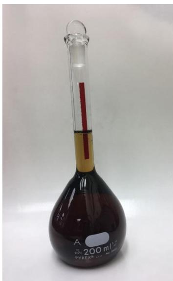
**Figure 4-9: Methylene Chloride Solution Prepared for Sonication**
