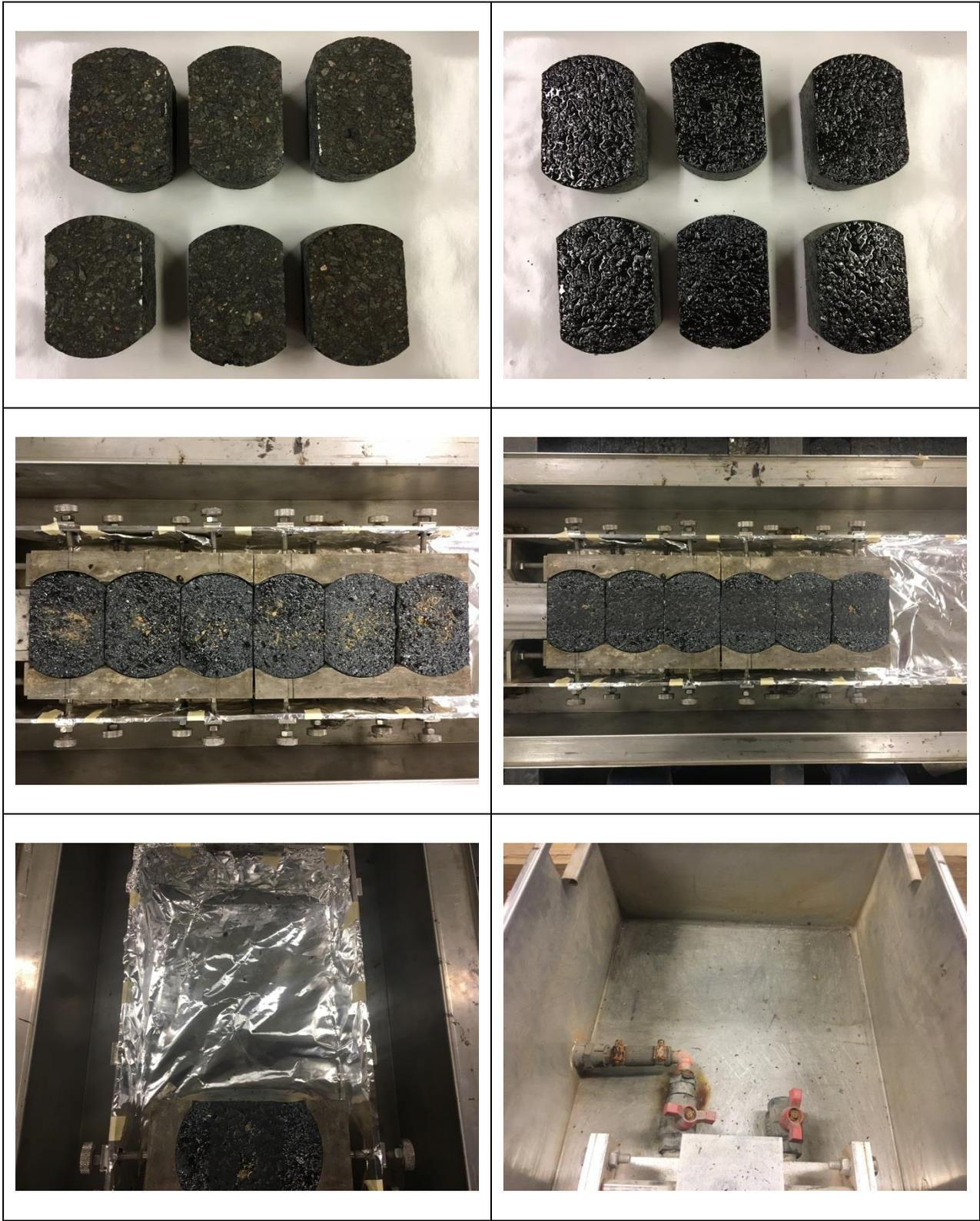
Figure C-8: Coal-Tar-Based, 48 Hour Cure Time, Sand Application, Test #1
