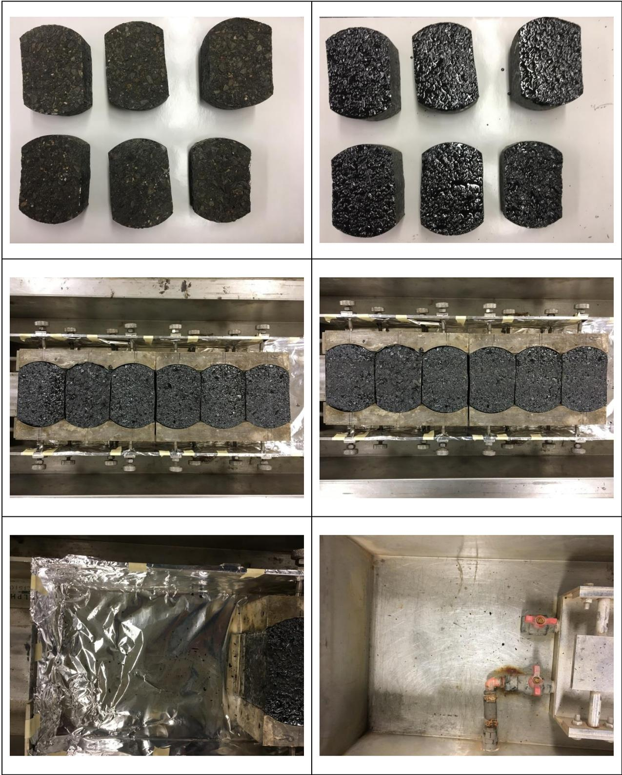
Figure C-6: Coal-Tar-Based, 3 Week Cure Time, Test #1
