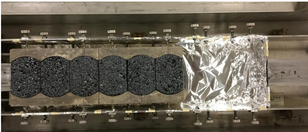
**Figure 4-2: Asphalt Discs Installed in MMLS with Aluminum Foil Liner**
