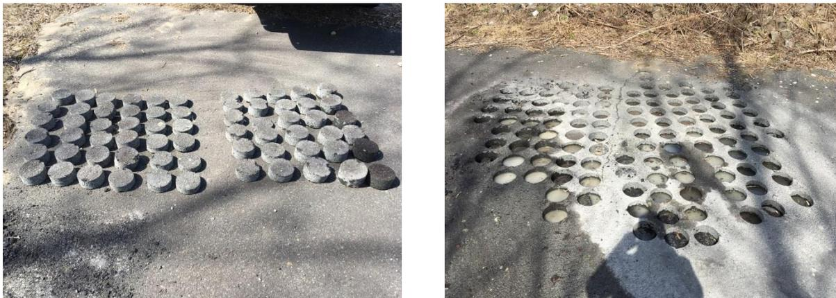
**Figure 4-6: Asphalt Cores from 3/28/ 2019 (Left) and All Asphalt Core Holes (Right)**
