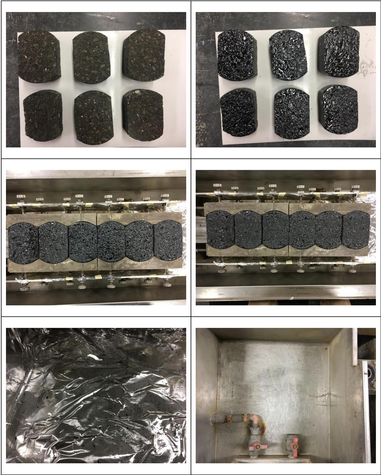
Figure C-4: Coal-Tar-Based, 48 Hour Cure Time, Test #2
