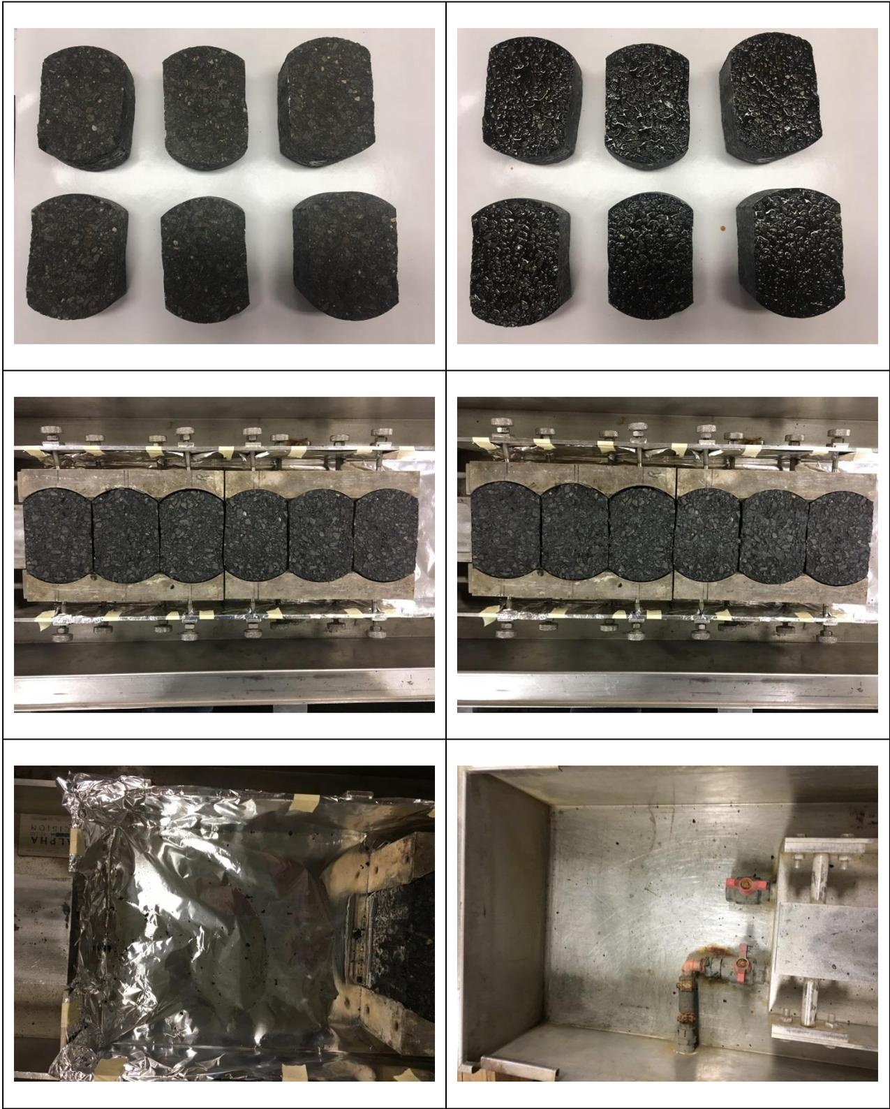
Figure C-13: Bio-Based, 3 Week Cure Time Test #2
