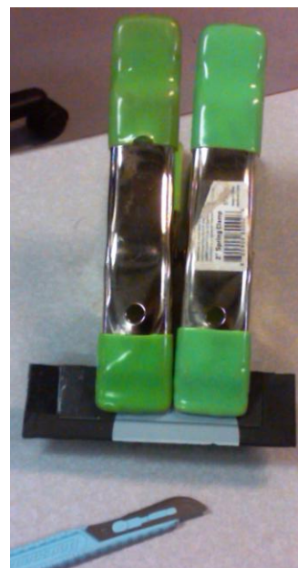
Figure 21: Scalpel and clamping system used for cutting samples
