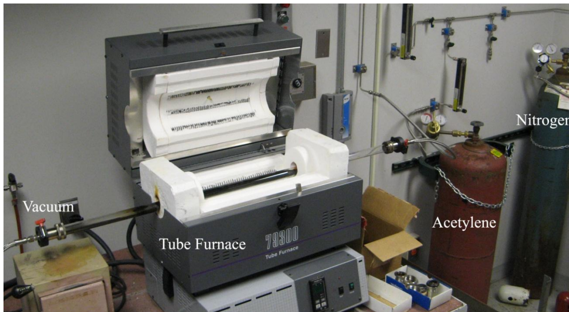
Figure 22: Tube furnace system used for chemical vapor deposition
