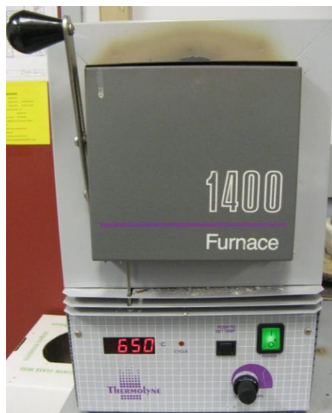
Figure 24: Furnace used for thermocleaning
