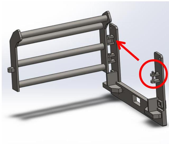
**Figure 28: Locking Pin Also Used to Hold Gate Open**
