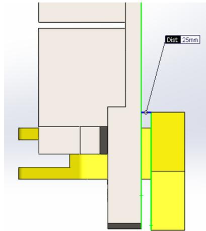
**Figure 32: Gap Between Rear Protection System Frame and Main Frame**
