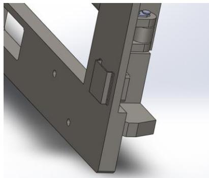
**Figure 30: Placement of Harness Protection Device on Frame**
