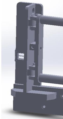
**Figure 18: Simple Pin Hold Open Mechanism**
