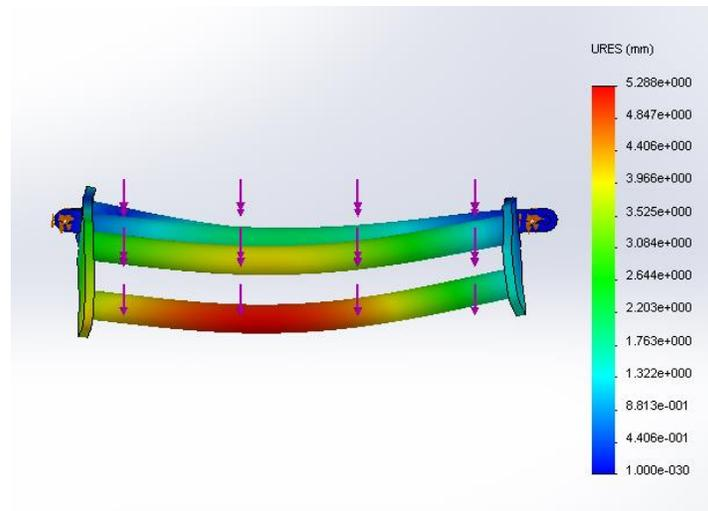
**Figure 37: Impact Displacement on Cross Bars**
