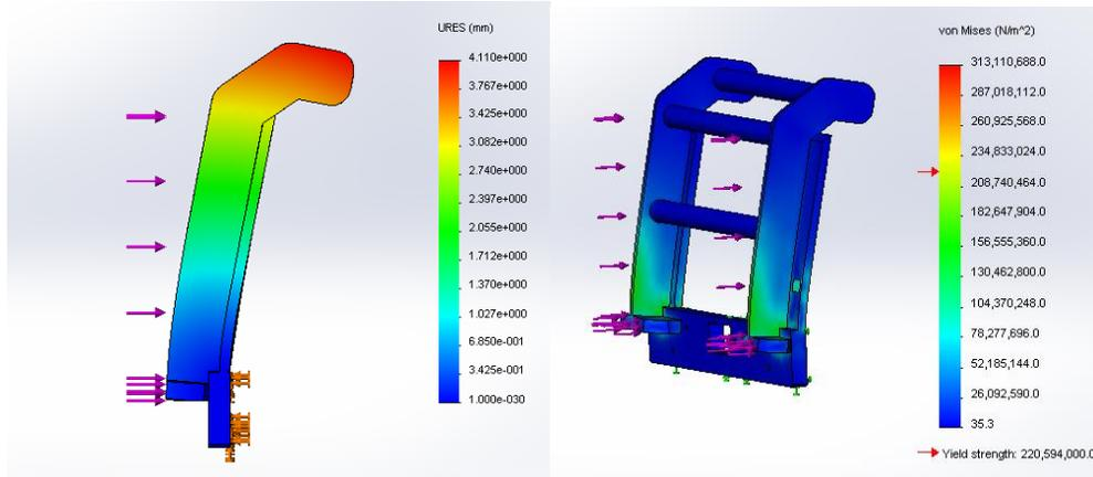
**Figure 21: FEM Analysis Second Iteration of Bend Uprights**
