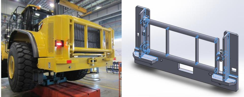
**Figure 6: Original Rear Protection Design (Picture and SolidWorks Model)**
