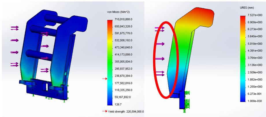
**Figure 20: FEM Analysis of the First Iteration of the Bent Upright Design**
