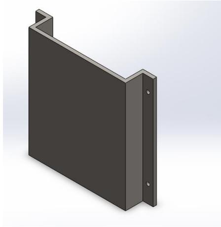
**Figure 31: Harness Protection Plate**
