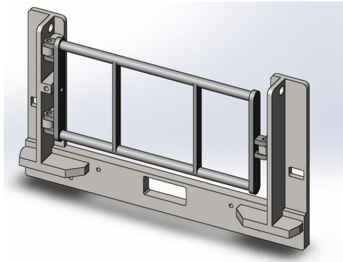
**Figure 17: Taller Design with Simple Pin**
