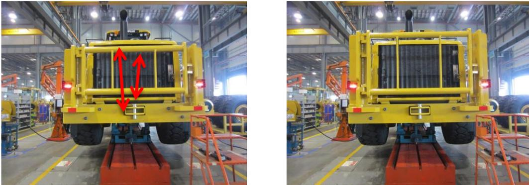
**Figure 13: Left Current Height of Gate, Right: Desired Height**
