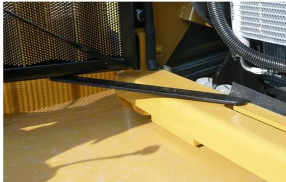
**Figure 11: Slider Hold Open Mechanism on Loader Radiator Guard**
