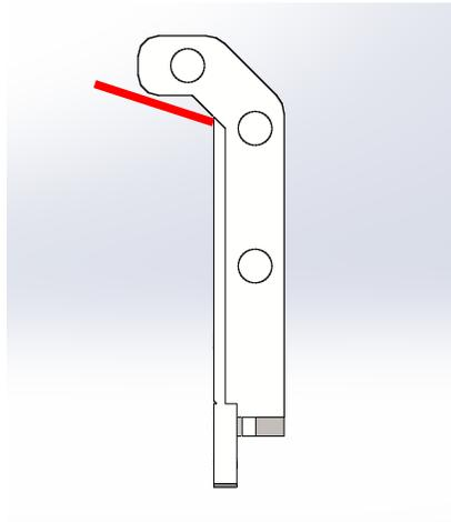
**Figure 26: Angle of Bend Upright Frame**
