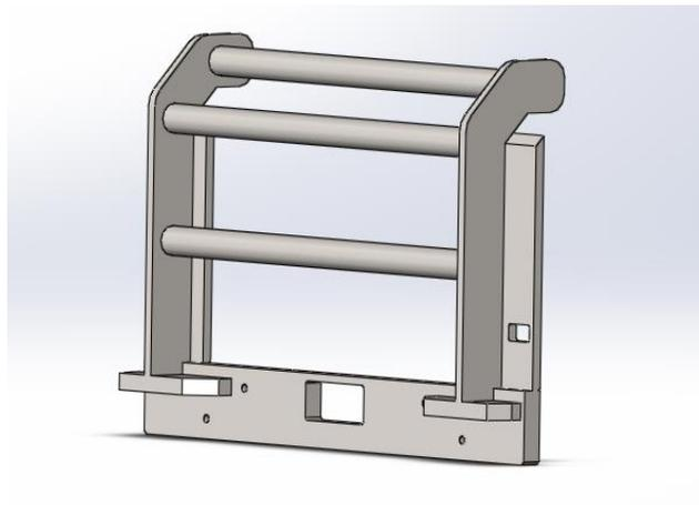
**Figure 22: Bent Upright Design**
