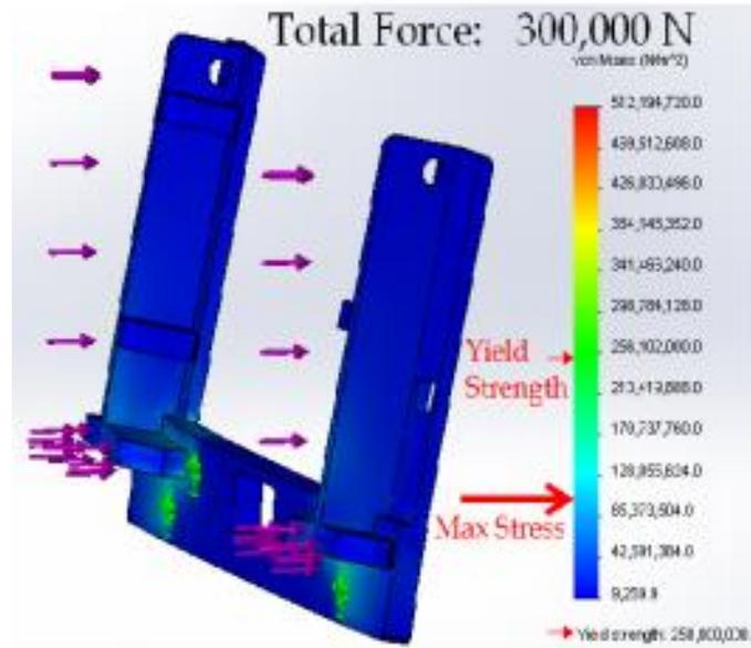
**Figure 8: Adjusted Frame Test**
