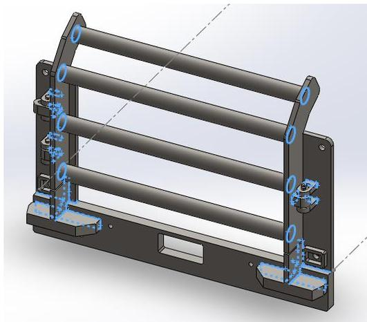
**Figure 42: Final Design Rear Protection Systems Weld Seams**
