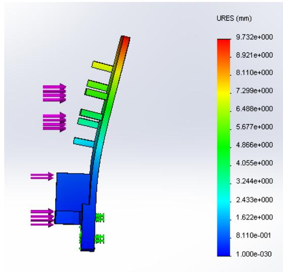
**Figure 35: Displacement of Frame**
