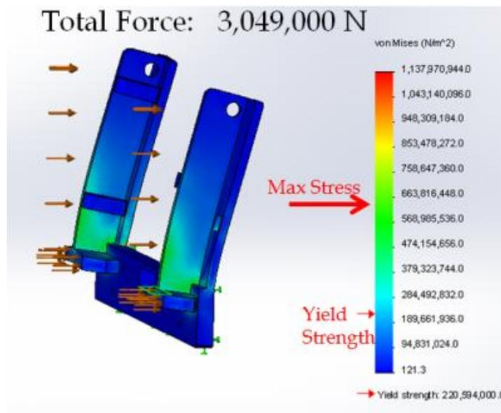
**Figure 7: Original Frame Collision Test**
