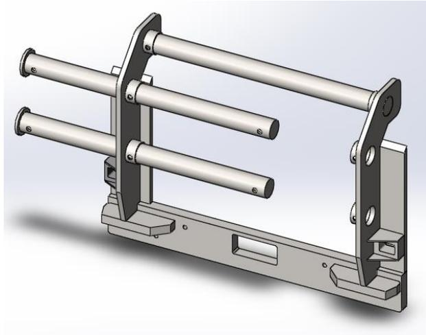
**Figure 23: Bend Upright Hold Open Mechanism**
