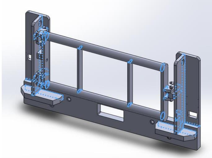
**Figure 41: Original Rear Protection Systems Weld Seams**
