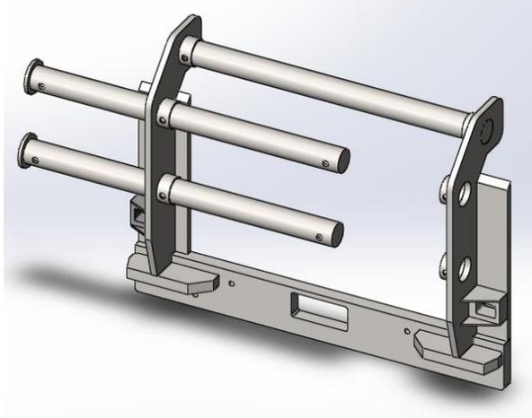
**Figure 16: Bent upright design**
