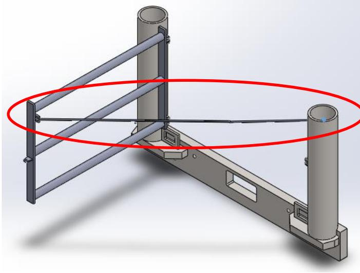
**Figure 16: Cylinder Uprights Hold Open Mechanism**
