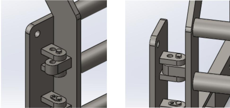
**Figure 29: Left: Closed, Right: Open**
