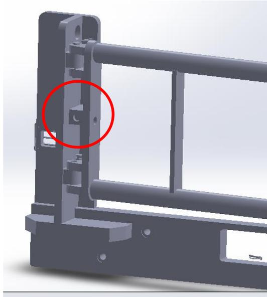
**Figure 14: Simple Pin Hold Open**
