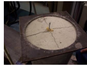
Figure 30: Concrete Failure, HY 150 Max Cleaned
