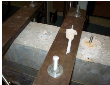
Figure 41: HIT HY 150 Max, Oversized, Wet Pull Out
