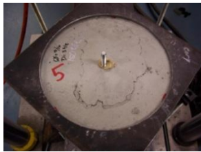
Figure 29: Concrete Failure, HY 150 Max Cleaned
