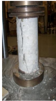
Figure 23: Concrete Cylinder Tested in Compression
