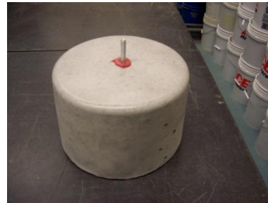
Figure 14: Sample with Installed Anchor
