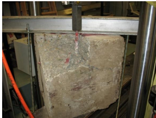
Figure 9: Preliminary Test 3: Concrete Edge Failure
