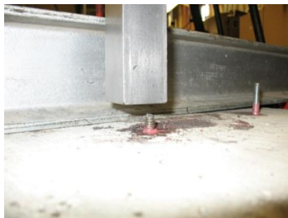
Figure 7: Failure of TZ anchor Test 1 and gripping fixture
