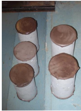
Figure 36: Capped Concrete Test Cylinders
