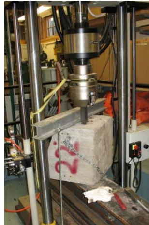
Figure 6: Preliminary Test 1: 3/8" TZ rods.
