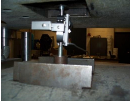
Figure 37: Attached Strain Gauge
