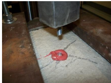
Figure 28: Ductile Steel Failure in Oversized HIT RE 500 Test
