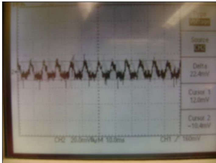
Figure 36: Output of +12V Regulator (20mV/div)
