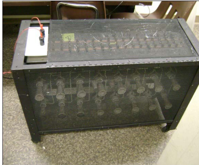
Figure 43: Resistor bank used for hall-sensor test
