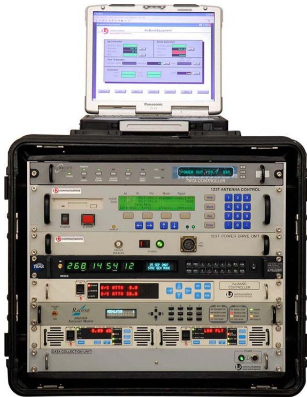
Figure 14: IMATE System Broadcasting Controls (Narda Satellite Networks).
