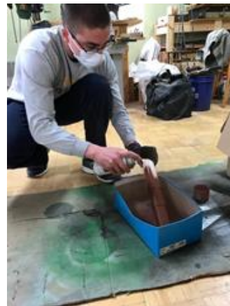
Figure 27. Spray Painting of PVC Pipes
