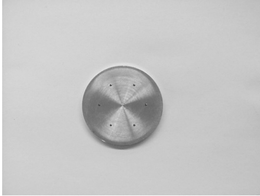
Figure 16 : Distributor stainless steel plate.
