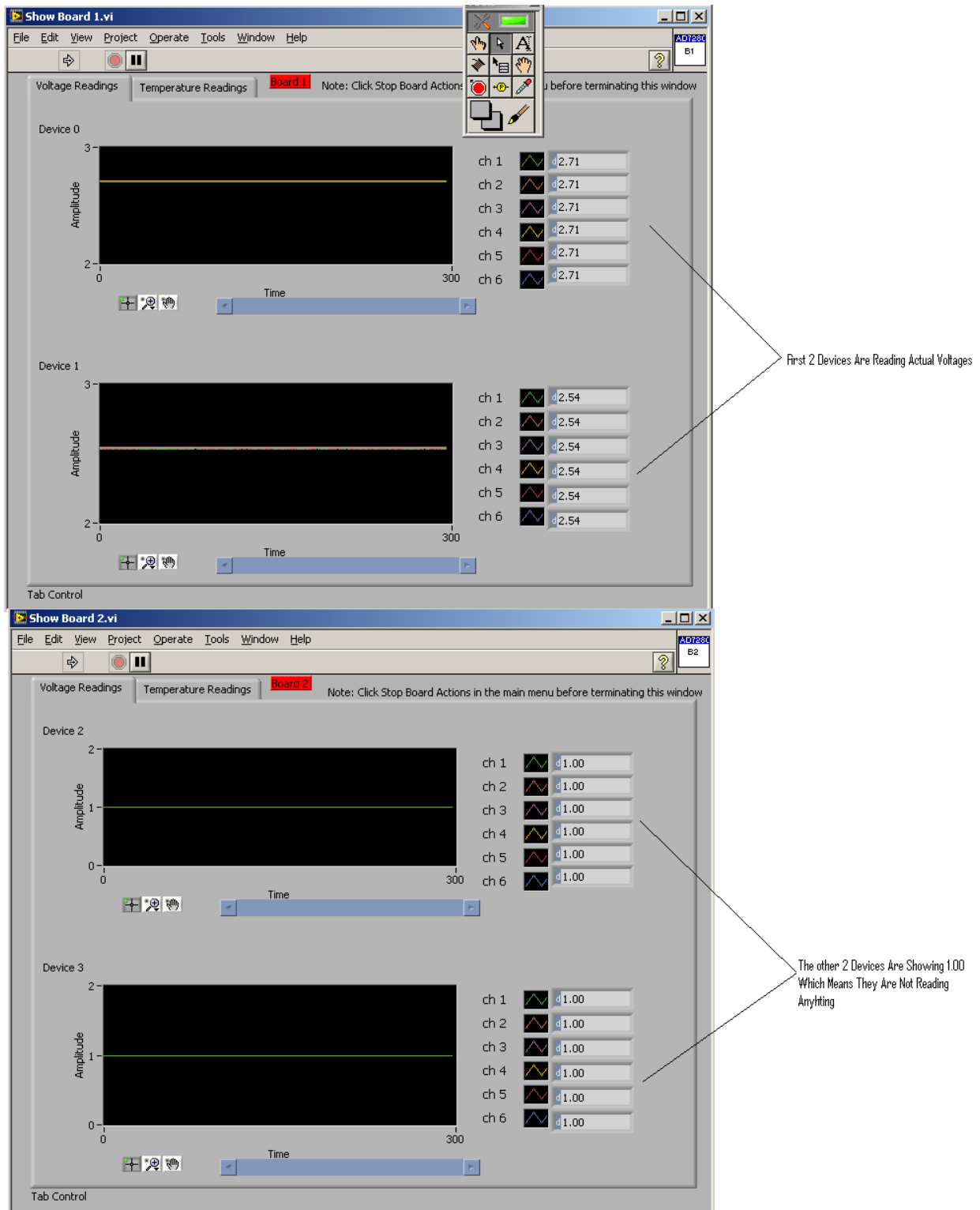
Figure 56 – Data from the master board (top) and the slave board (bottom). Note that the slave is not receiving data.
