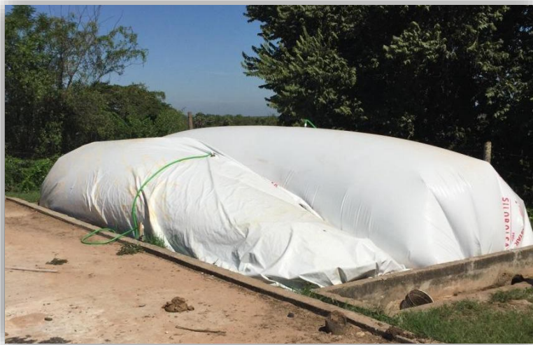
Figure 5: Old Biodigester System
