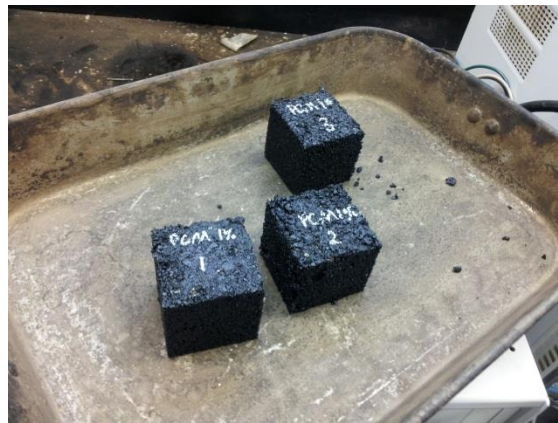
Figure 16: Compacted HMA samples with 1.25% PCM-6.
