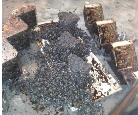
Figure 17: Samples with 10.5% PCM-6 after demolding.
