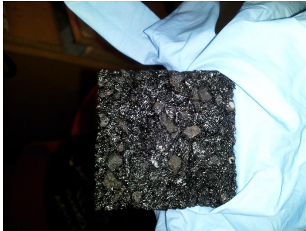
Figure 18: Observed difference in color shading on faces of cubes with 2.5% PCM-6.
