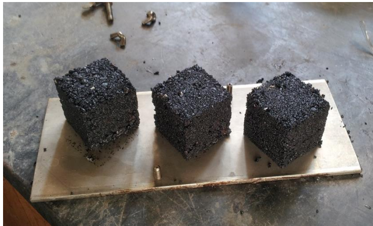
Figure 25: Phase 3 batch of 1.25% PCM-6 samples after demolding.
