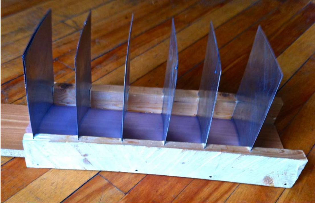
Figure 36: Silicone thickness testing device.
