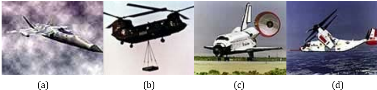
Figure 7: (a) Short-Takeoff/Vertical-landing Fighter, (b) Helicopter, (c) Space Shuttle, and (d) The Tiltrotor [3]
