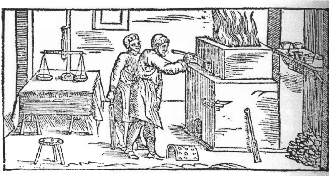
Fig. Cupeling hearth with cupels, muffle, and balance for the assay. 15
