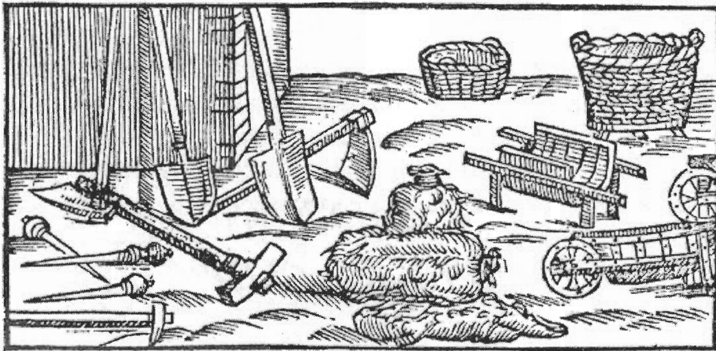
Fig. Mining tools. Picks, shovels, baskets, barrows. 10
