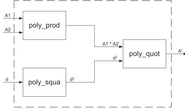
Figure 6.4: Block diagram of the calculation of  $A'(u)$
