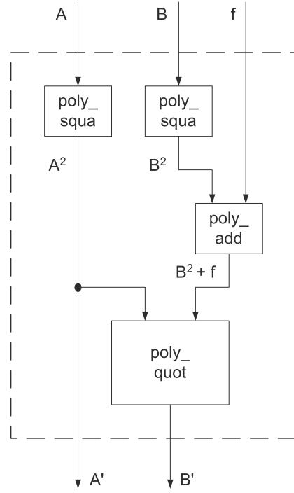
Figure 6.8: Block diagram of doubling
