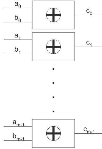
Figure 4.1: Addition in  $GF(2^m)$
