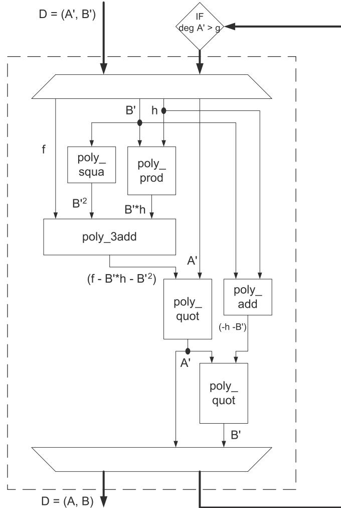
Figure 6.7: Block diagram of the design of the Gauss Reduction Algorithm
