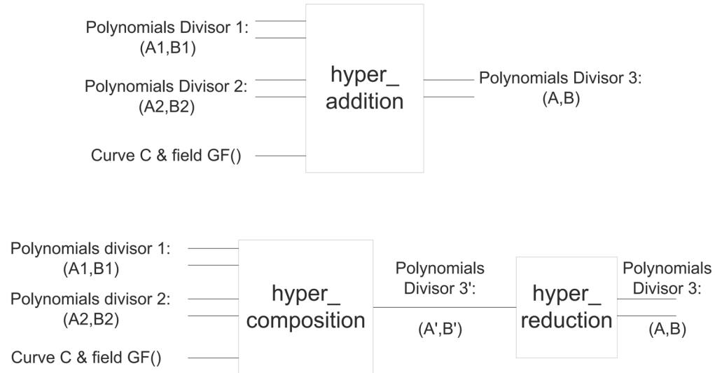
Figure 6.1: Block diagram for addition on Hyperelliptic Curves
