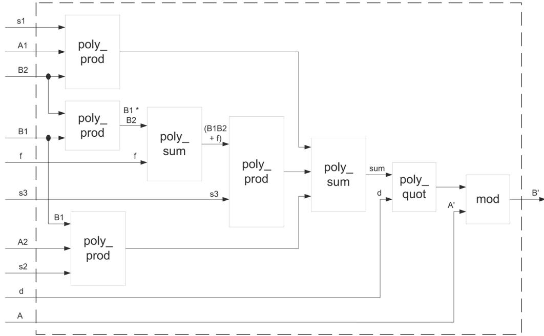
Figure 6.5: Block diagram of the calculation of  $B'(u)$
