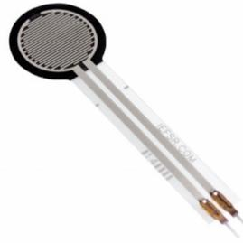
*Figure 8: Force Sensitive Resistor*
