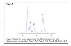
distinct peaks as shown in figure 4. Peaks 1 and 2 correspond to the R isomer. Peak 1 represents R,R and Peak 2 represents R,S. Peaks 3 and 4 correspond to the S isomer, in which Peak 3 is S,S and Peak 4 is S,R.
