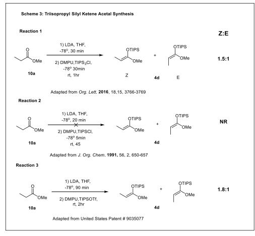
each method would perform when used to functionalize chromenones (see Appendix 1D for procedure). The silyl ketene acetal from Reaction 3 functionalized the chromenone with more diastereocontrol than the silyl ketene acetal from Reaction 1 could achieve (Table 2, Reaction 1 and 3). Therefore, **4d** for the following investigations was synthesized using the method as described in Reaction 3 (Scheme 3).
